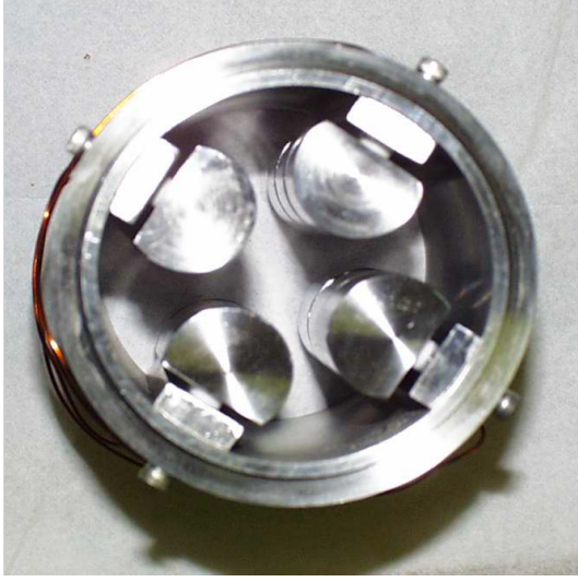
(a) Top view of the linear Paul trap. Picture taken from [57].
