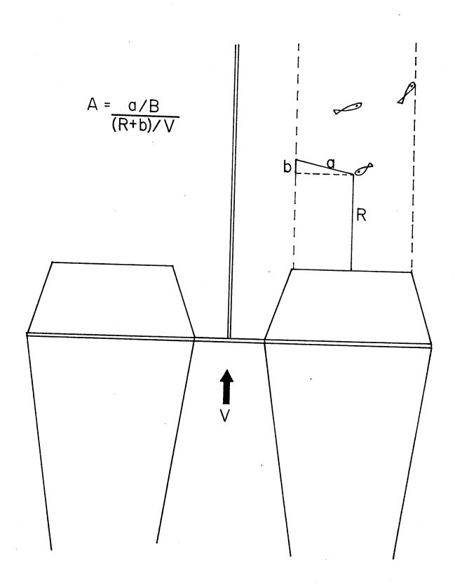
Figure 23. Avoidance calculation fitted to shiner density estimates using an escape route angle of  $85^{\circ}$ .
