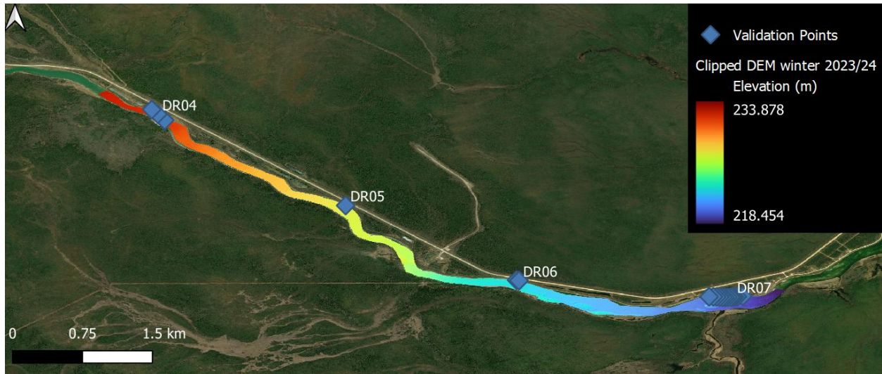
Figure 14. Clipped DEM of Winter 2023/24 with 18 top-of-ice elevation points used for accuracy validation.
