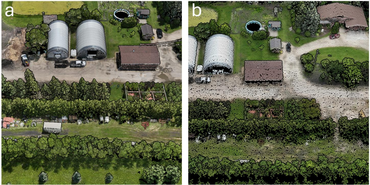
Figure 15. A visual illustration of the difference between high and low-density point clouds. (a) high-resolution point cloud; (b) generated point cloud using the low-resolution setting.
