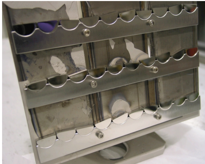
Figure 10: Sample jig used to hold 30 samples at a time for the deposition process.
