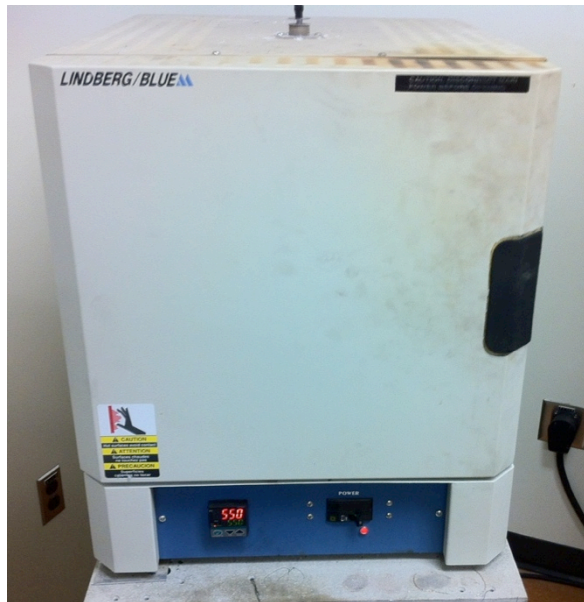
Figure 15: Blue M box furnace used for oxidation of samples at 1100 °C.
