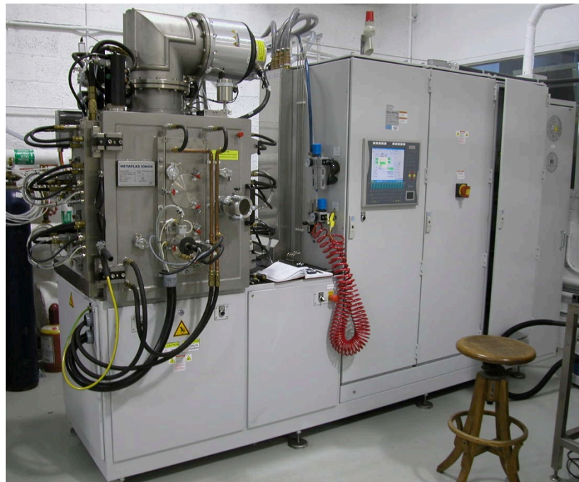
Figure 12: Sulzer Metaplas MZR304 CAD equipment used for deposition of the Ni-5Cr-15Al overlay coating.
