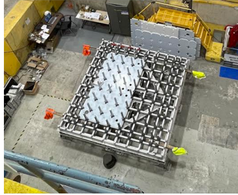
Figure 2.15: MSR's base with supporting Al extrusion.
