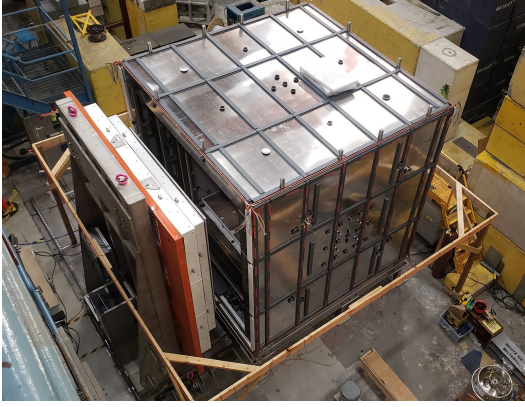
Figure 2.20: MSR's \mu -metal layers.
