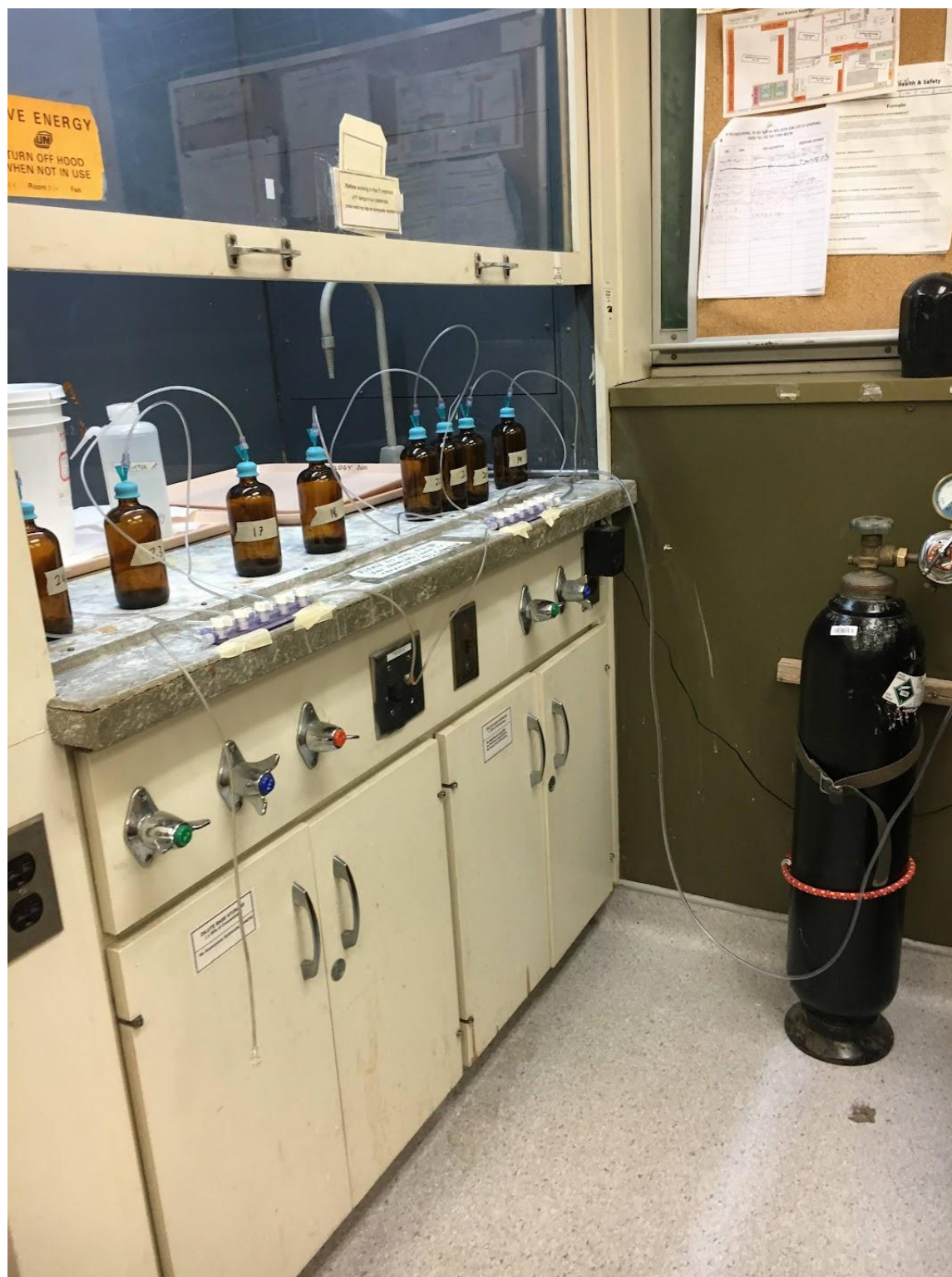
Figure 3.10. Nitrogen gas injection apparatus for filling Boston rounds with nitrogen gas.
