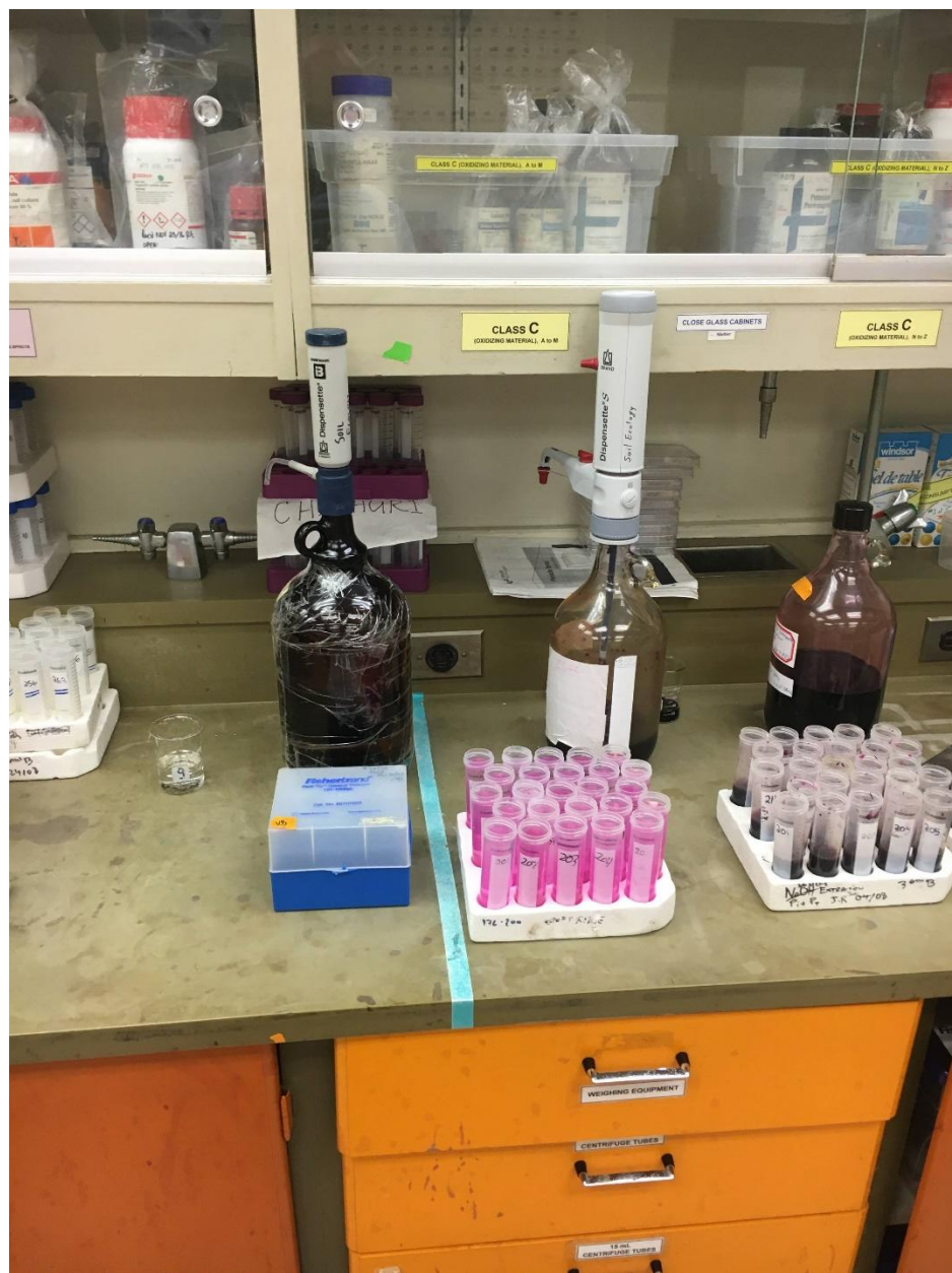
Figure 3.8. Image of diluted supernatant for active carbon analysis.
