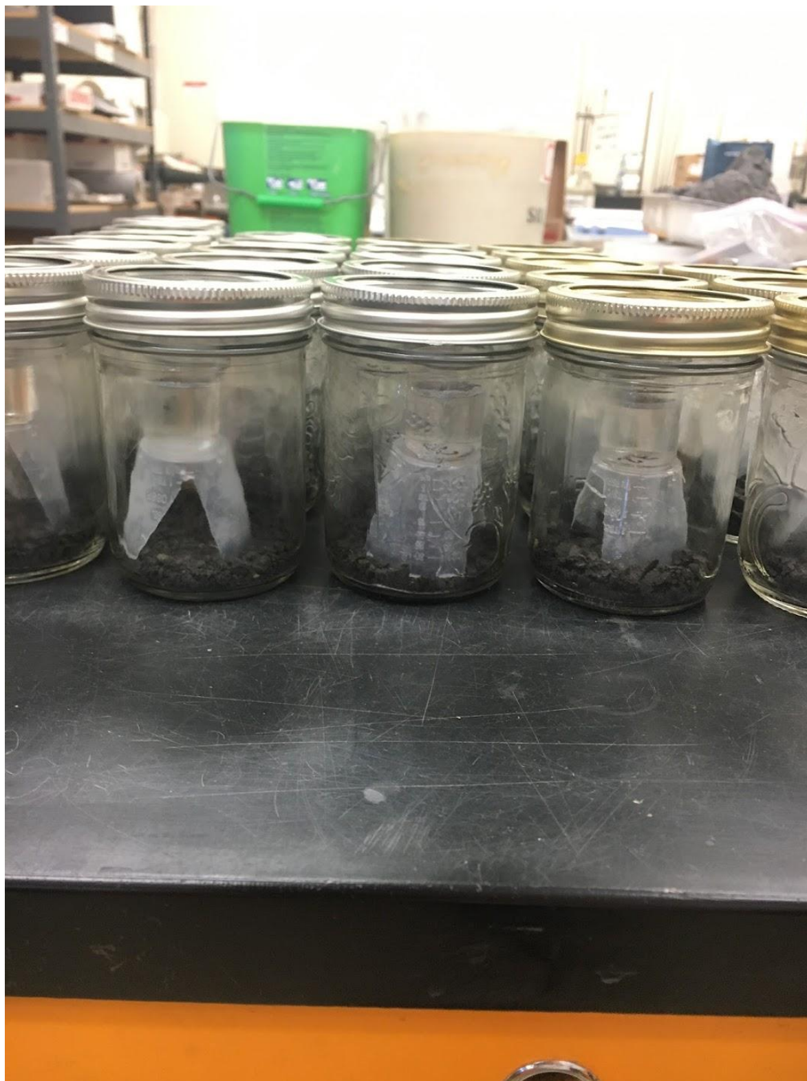
Figure 3.11. Jars containing soil and potassium hydroxide trapping solution used in soil respiration test.
