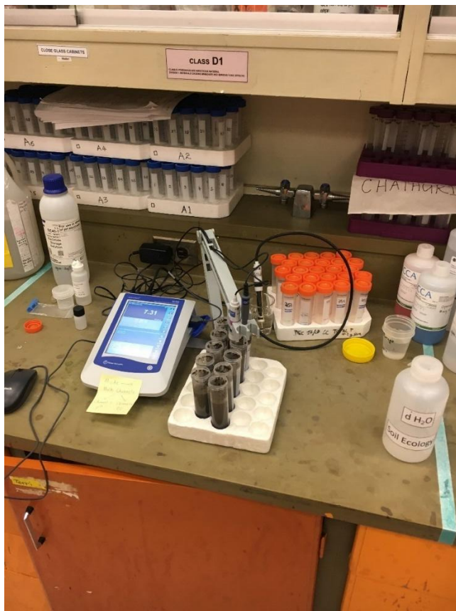
Figure 3.12 Image of pH meter testing soil slurry.
