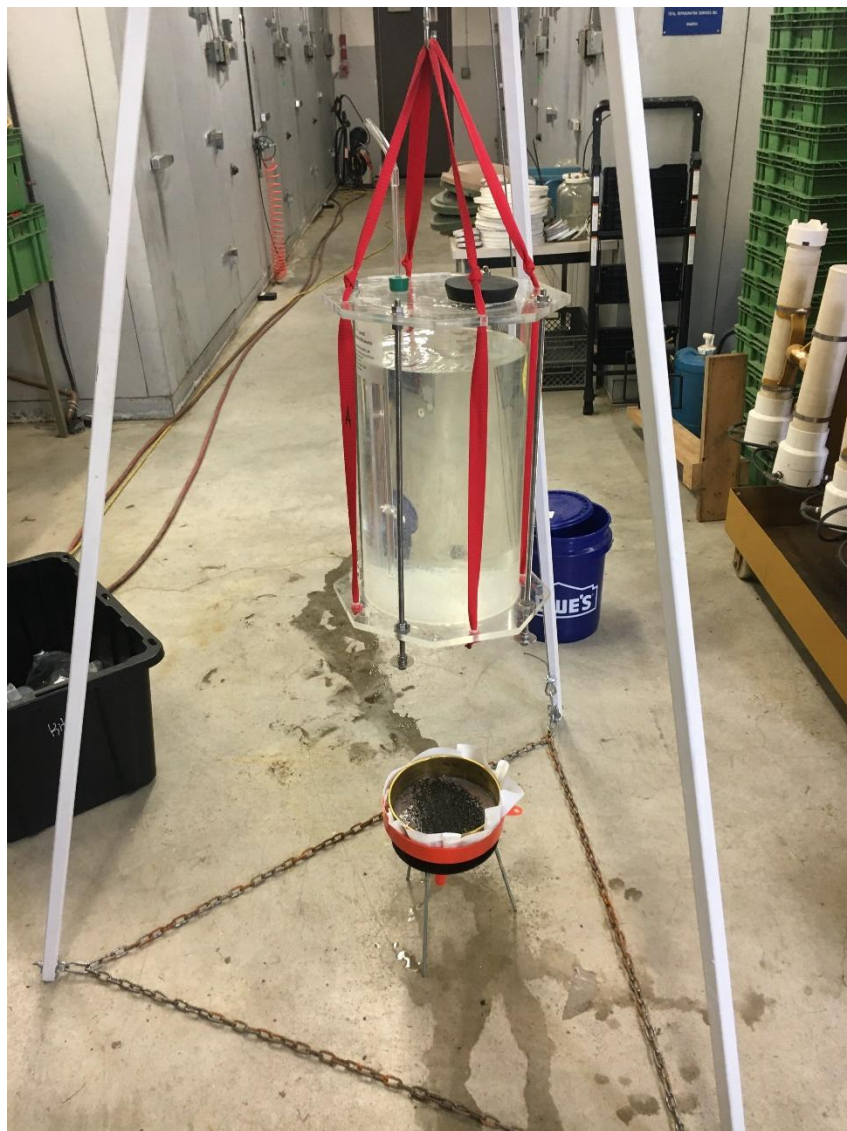
Figure 3.7. Wet aggregate stability testing equipment consisting of a Cornell infiltrrometer suspended above soil on 0.25 mm sieve that is sitting on a funnel and trivet.
