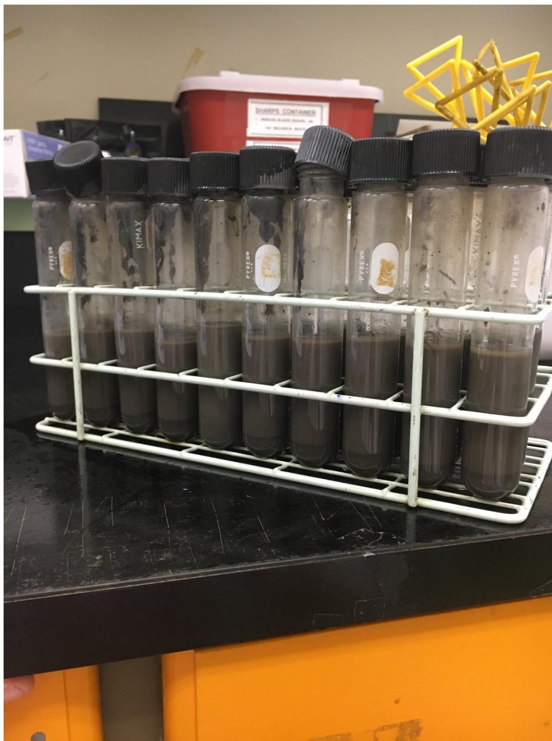
Figure 3.9. Soil and citrate slurry in test tubes after autoclave treatment.
