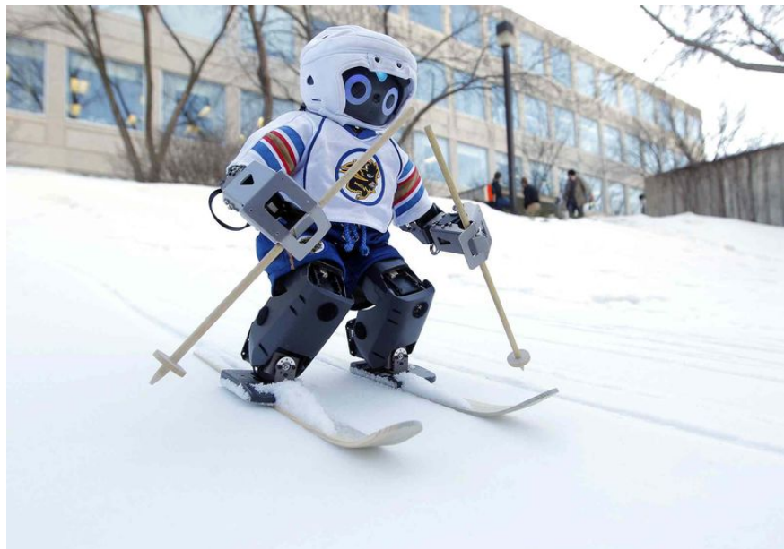
Figure 6.1: Jennifer the robot equipped with skis demonstrating alpine skiing. We use the Do the Shake policy to control the robot’s pitch and roll while skiing. This skiing research won the 2015 ICRA Humanoids Application Challenge. (Winnipeg Free Press [30])
