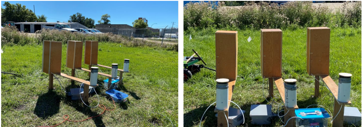
Fig. 4.5 In-Field setup and wiring of a plant-controlled atmometer
