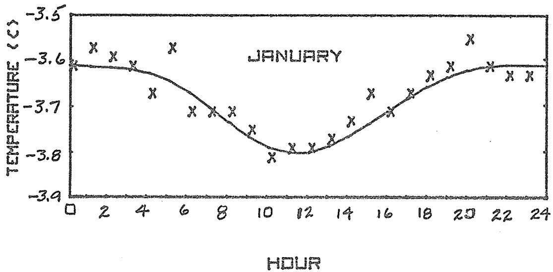
Figure 6. Observed average diurnal soil surface (1 cm) wave (x) at WNRE for January (1968-1973) and best-fit Fourier-series curve (solid line).
