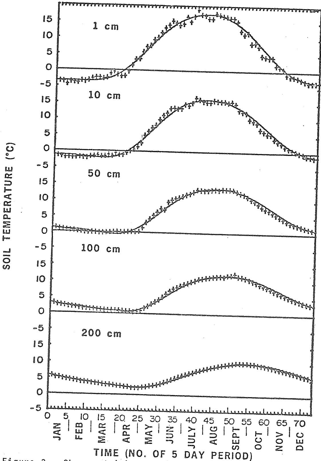
Figure 3. Observed (+) average annual soil temperature waves at five levels at WNRE (1968-1972) and best-fit Fourier-series curves (—).
