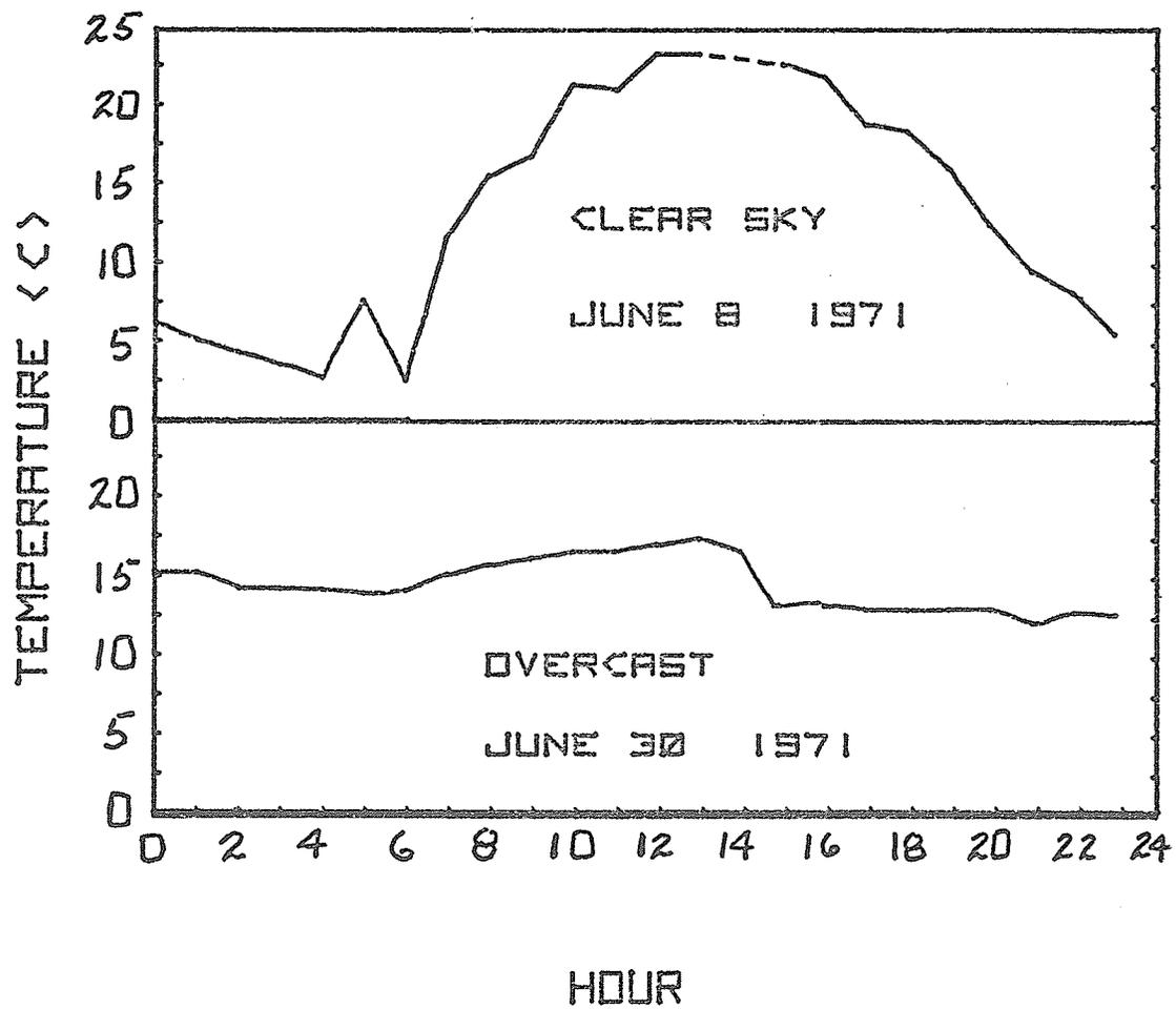
Figure 5. Observed soil surface (1 cm) temperature fluctuations on a clear day and on a cloudy day at WNRE (the sudden cooling at mid-afternoon on June 30 is not typically diurnal).
