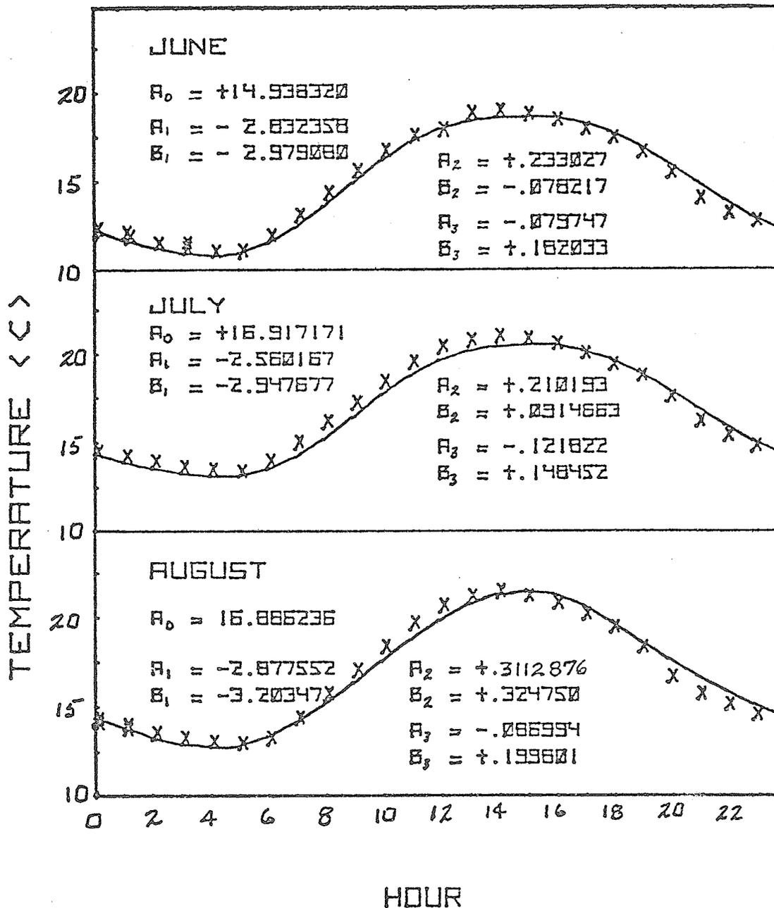
Figure 4. Observed (X) average diurnal soil surface (1 cm) temperature waves for June, July and August (1968-1972) and best-fit Fourier-series curves (solid line) at WNRE.
