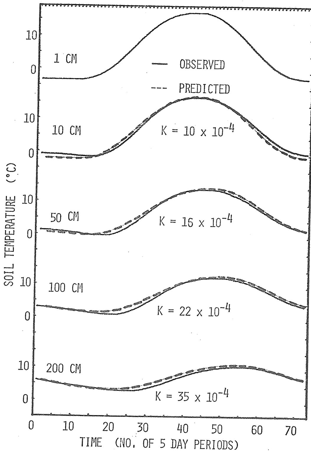
Figure 16. Observed and predicted subsoil annual temperature waves from Equation (37).
