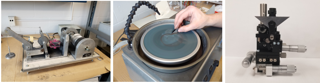
Figure 3.8: A series of images showing the fabrication of the ATR prism. The image on the left shows the prism being cut from a block of HRFZ Si, while the middle image shows polishing of the prism. The image on the right shows final prism mounted in a 3 axis stage.
