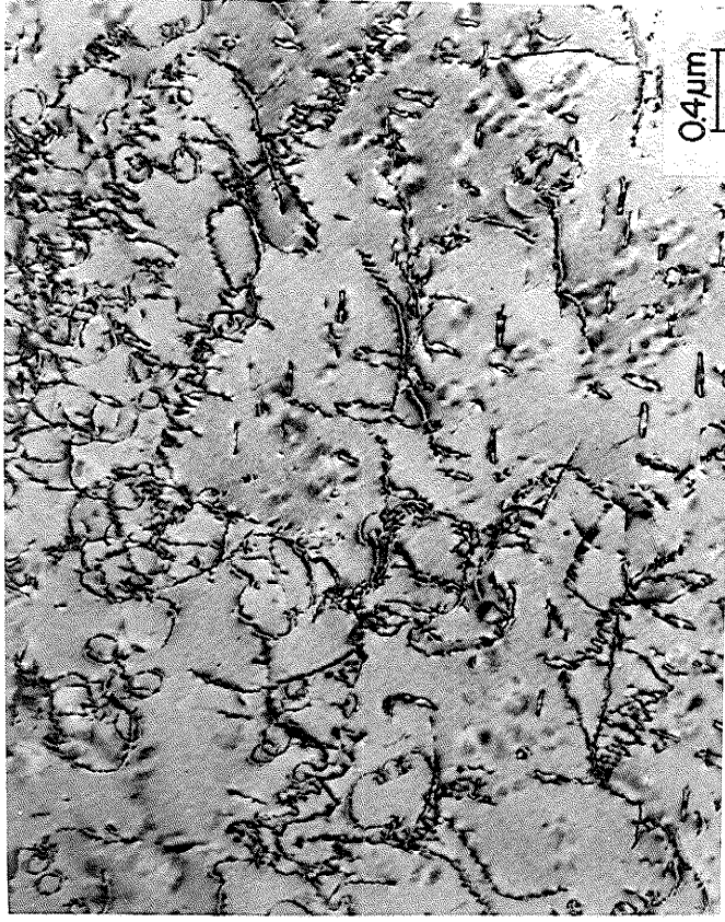
Fig. 4.6 Bright field image of the Al-1.53%Cu-0.79%Mg alloy aged at room temperature for 48 h and further aged at 130°C for 600 h
