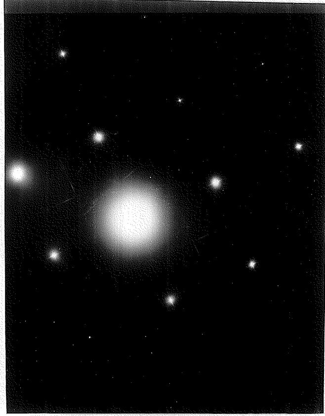
Fig. 5.31 (a) Bright field image of the Al-1.52%Cu-0.77%Mg-1.03%Si alloy aged at room temperature for 48 h and further aged at 190°C for 24 h (b) SAD pattern of (a)
