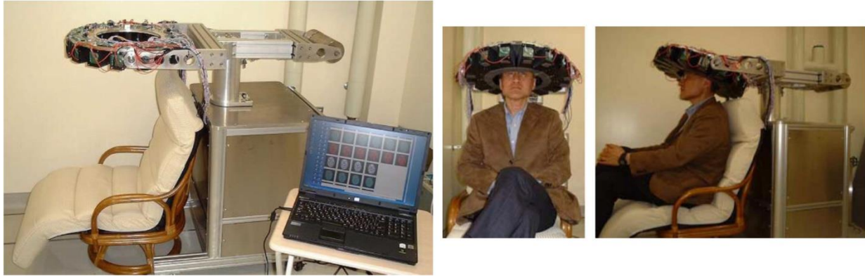
Figure 2.19. The PET-hat system (left) and the PET-hat with a subject (middle and right) © 2011 IEEE [115].
