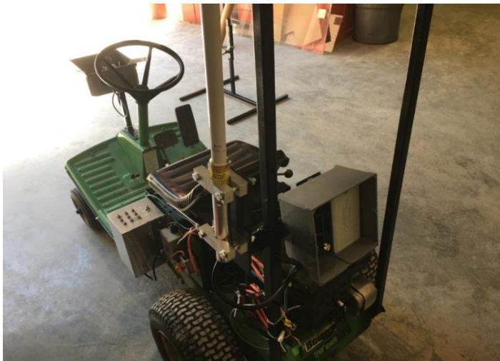
Figure 11: View of mower from back, with radio and antenna mounted.
