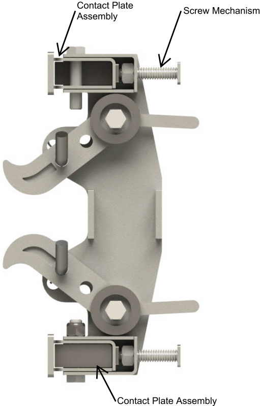
Figure 19: Impeller clamp contact plate assembly.
