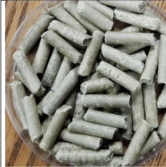
Figure C. 17 Miscanthus pellet made at low temperature (maximum 80 °C) and 30% particle moisture content(wb) no additives added.
