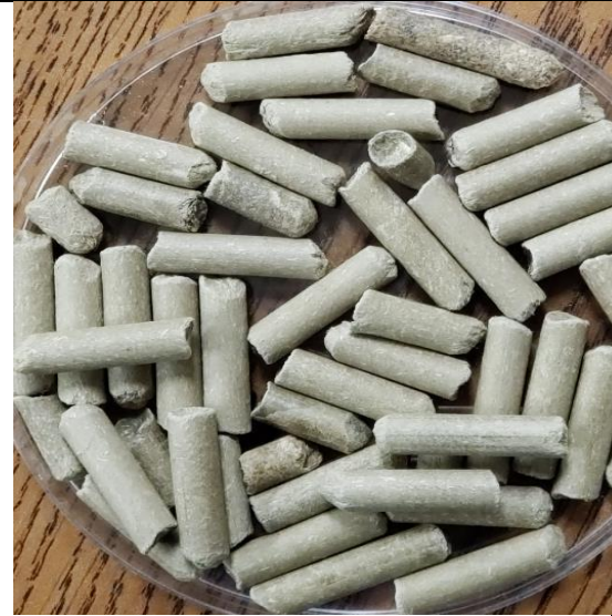
Figure C. 18 Prairie chord grass pellet made at low temperature (maximum 80 °C) and 30% particle moisture content(wb) no additives added.
