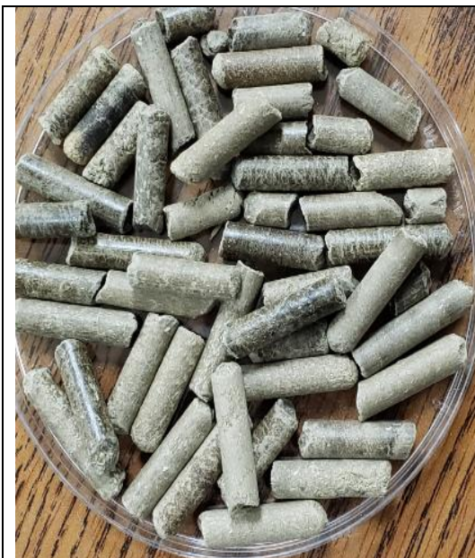
Figure A. 19 Switch grass pellet made at low temperature (maximum 80 °C) and 30% particle moisture content(wb) no additives added.
