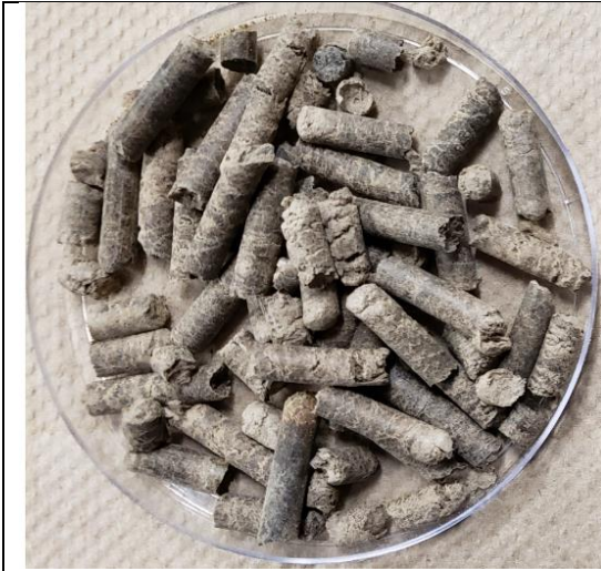
Figure A. 5 Paper towel pellet made at low temperature and 25% particle moisture content(wb).
