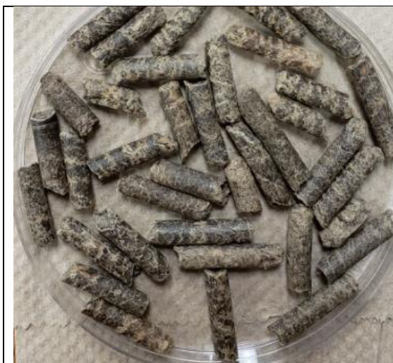
Figure B.15 Paper box pellet made at low temperature and 35% particle moisture content(wb) with no additives added.
