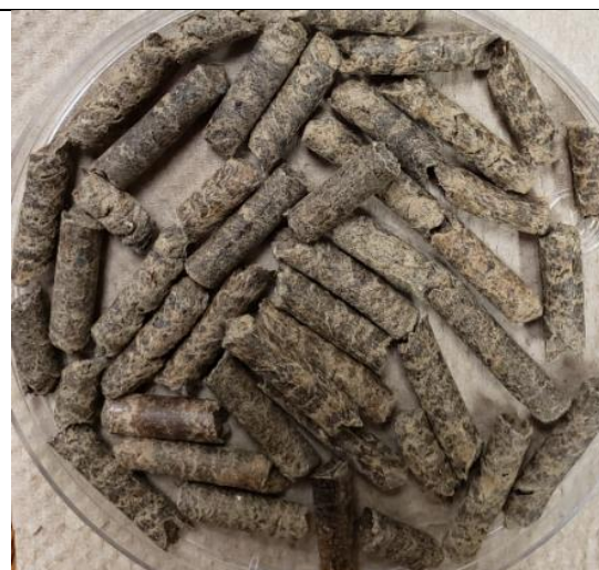
Figure B. 16 Paper box pellet pellet made at low temperature and 35% particle moisture content(wb) with yeast as additives.
