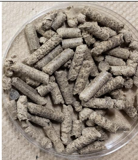
Figure A. 8 Paper towel pellet made at high temperature and 30% particle moisture content(wb).
