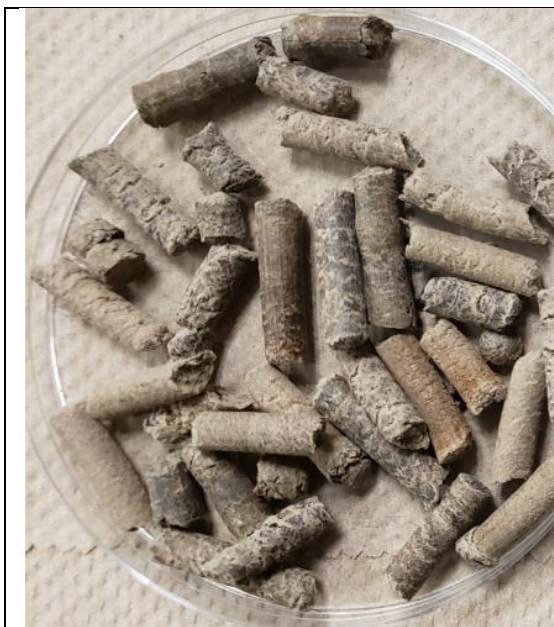
Figure A. 13 Paper towel pellet made at low temperature and 55% particle moisture content(wb).
