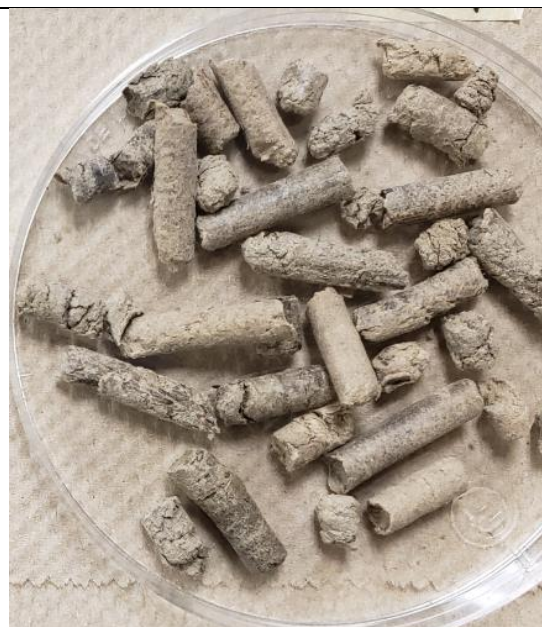
Figure A. 14 Paper towel pellet made at high temperature and 55% particle moisture content(wb).
