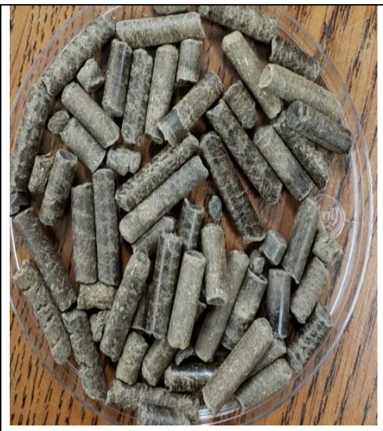
Figure A. 20 Big blue stem pellet made at low temperature (maximum 80 °C) and 30% particle moisture content(wb) no additives added.
