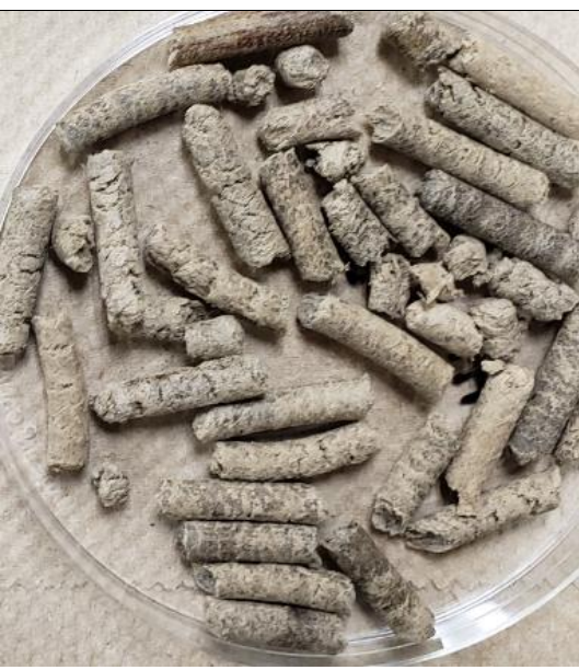
Figure A. 12 Paper towel pellet made at high temperature and 45% particle moisture content(wb).
