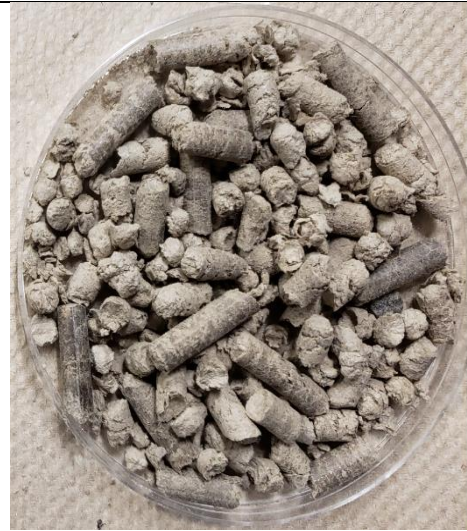
Figure A. 6 Paper towel pellet made at high temperature and 25% particle moisture content(wb).
