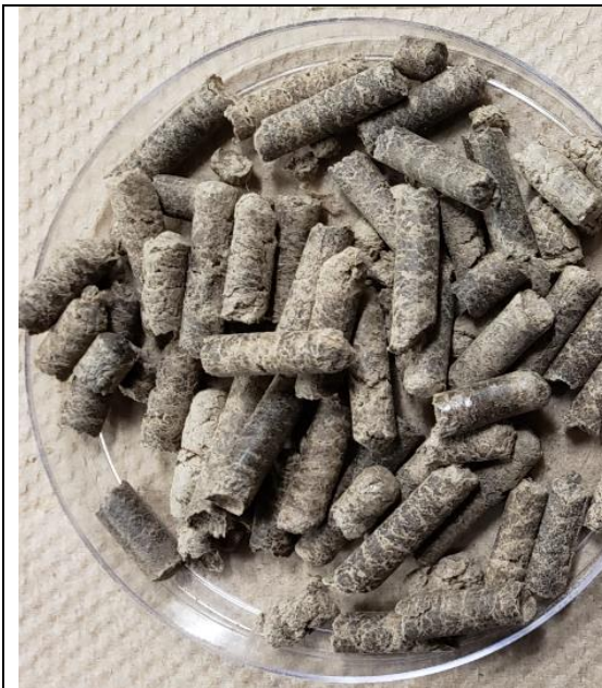
Figure A. 7 Paper towel pellet made at low temperature and 30% particle moisture content(wb).
