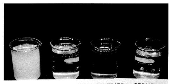
FEED WATER FILTERED CONCENTRATE PERMEATE
