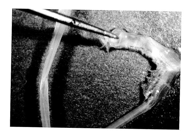
Figure 4.5. Iodine reaction to UF fouling layers.
