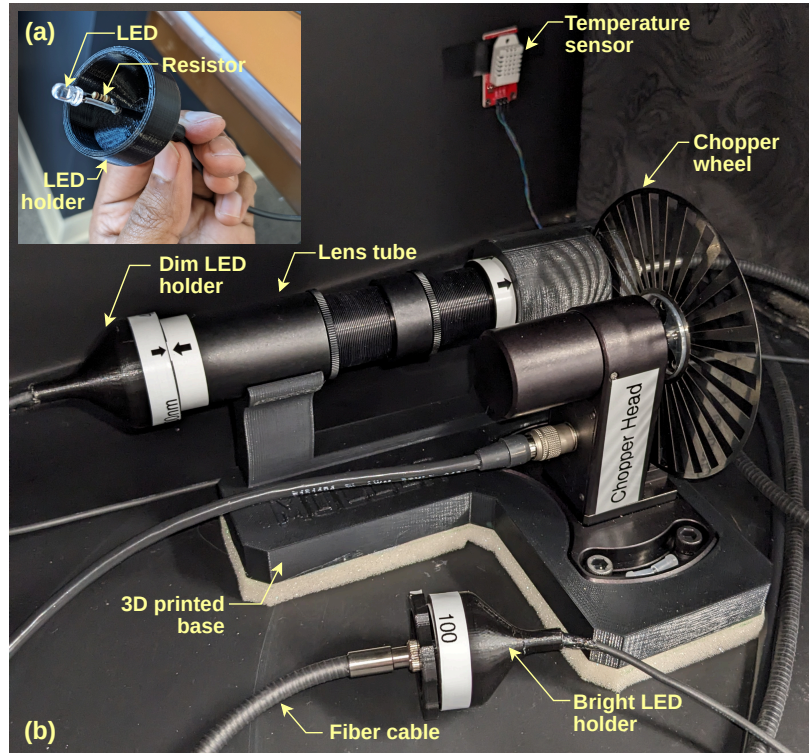
Figure 2.4: (a) An LED attached to the holder (LED is pushed outward otherwise usually sits at the back of the holder), (b) Complete chopper wheel apparatus.
