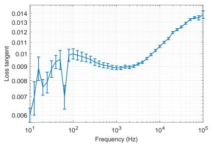
(b) Mean value of the loss tangent is plotted and error bars show the standard error of the mean loss tangents values.
