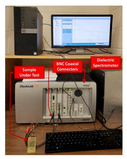
**Fig. 6.8:** Test samples connected to the dielectric spectrometer for measurements of capacitance and dielectric loss. Sample is connected to the device via BNC coaxial cables.
