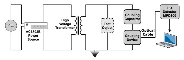
**Fig. 6.25:** PD test setup block diagram. Sample under the test is connected to a high voltage transformer which is fed through a digital adjustable power supply.
