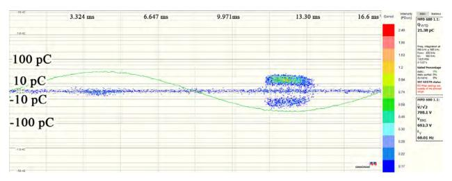
Fig. 6.29: Phase resolved PD pattern for a 20 cycle aged single coated test board with ENIG surface finish.
