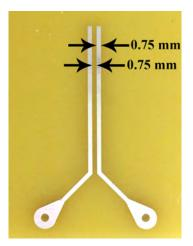
Fig. 4.1: Y shape layout test board for PD under pollution and breakdown voltage tests based on IPC-TM-650. The board size was 35 mm by 45 mm and the clearance of parallel tracks and the width of traces are both  $750 \text{ }\mu\text{m}$
