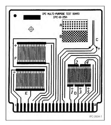
**Fig. 2.3:** IPC multi-purpose test board IPC-B-25A. Including "Y" shape, "D", "E", and "F" comb patterns [12].
