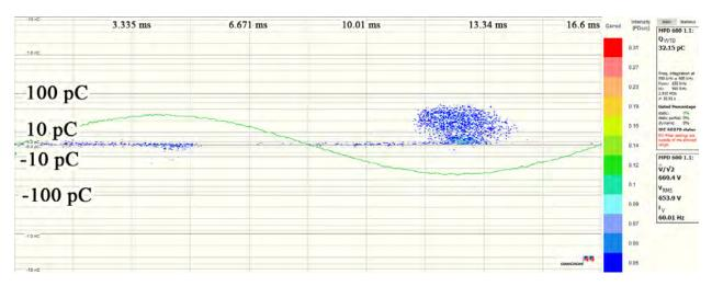
**Fig. 6.32:** Phase resolved PD pattern for a 36 cycle aged single coated test board with HASL surface finish.
