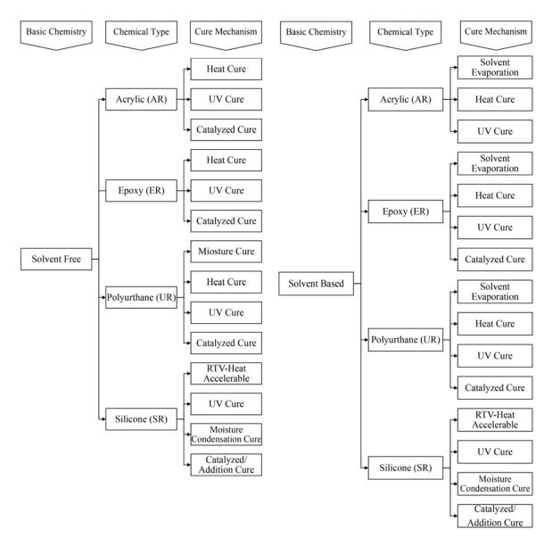
Fig. 2.1: Conformal coating materials family tree based on IPC-HDBK-830 [17].
