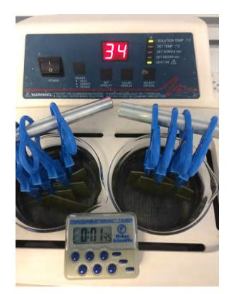
Fig. 4.3: Cleaned plastic clips hung from aluminum bars are holding the samples in ultra sonic bath of Ammonia solution at  $35 \pm 1$  °C.
