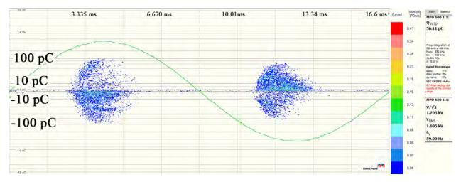
**Fig. 6.27:** Phase resolved PD pattern for a 20 cycle aged double coated test board with ENIG surface finish.
