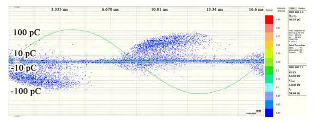
Fig. 5.7: Phase resolved PD pattern for coated PCBs with aluminum particles on top.
