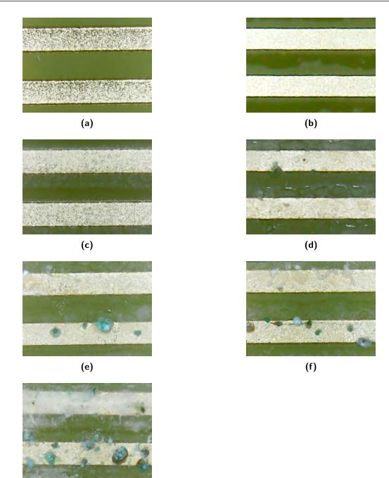
**Fig. 6.7:** Macro imaging with 360 X magnification from traces of test boards with ENIG finish which have degraded during 36 cycles of thermal and humidity aging under energized condition: a) new sample, b) 1 cycle aged, c) 4 cycles aged, d) 7 cycles age, e) 10 cycles aged, f) 20 cycles aged, g) 36 cycles aged.
