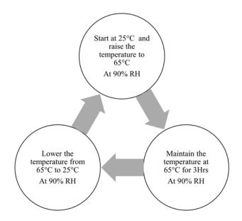
Fig. 6.1: Thermal and humidity aging cycles sequence diagram.
