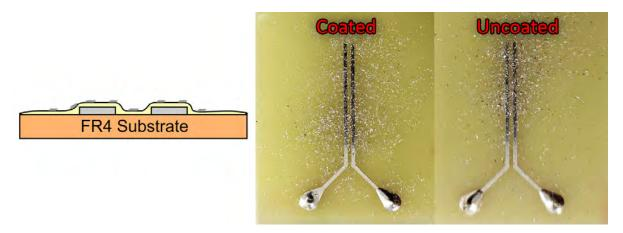
**Fig. 5.4:** Coated and uncoated test boards with aluminum particles distributed evenly on top.
