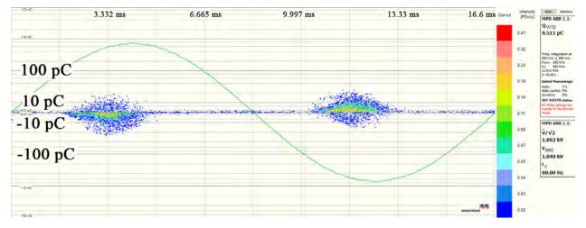
Fig. 6.28: Phase resolved PD pattern for a 20 cycle aged double coated test board with HASL surface finish.
