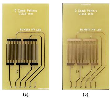
**Fig. 4.2:** Standard D comb pattern test samples. Clearance between conductors and width of each trace of the comb lines are equal to 0.315 mm. a) Test board with HASL surface finish, b) Test board with ENIG surface finish.
