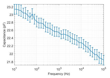
(a) Mean value of the capacitance is plotted and error bars show the standard error of the mean capacitance values.
