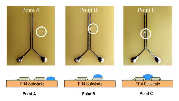
**Fig. 5.3:** Coated test board with saltwater drop on three different selected locations and the illustrate of cross section of the samples.
