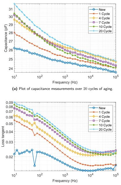
(b) Plot of loss tangent measurements over 20 cycles of aging.
