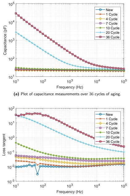
(b) Plot of loss tangent measurements over 36 cycles of aging.
