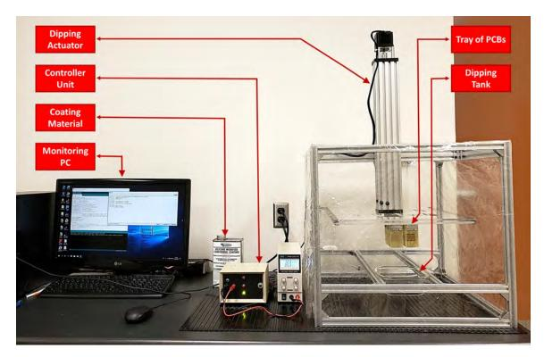
**Fig. 4.5:** Conformal coating application device with controlled speed that was designed and developed in McMath High Voltage Lab. The micro-controler unit adjusts the actuator speed and send the system report to PC. Boards are mounted on a tray, ready for dipping in a tank of silicone coating polymer.
