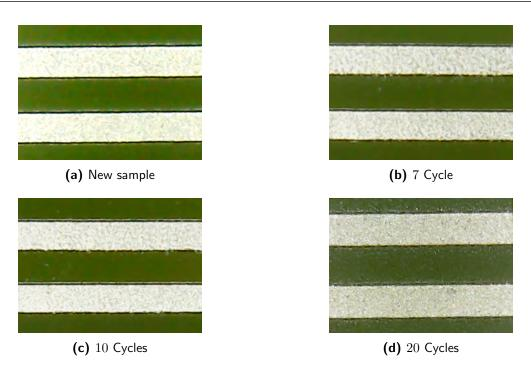
**Fig. 6.15:** Macro imaging from traces of single coated test boards with ENIG finish which have degraded during 20 cycles of thermal and humidity aging under non-energized condition.
