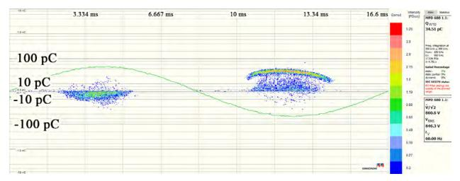
**Fig. 6.30:** Phase resolved PD pattern for a 20 cycle aged single coated test board with HASL surface finish.
