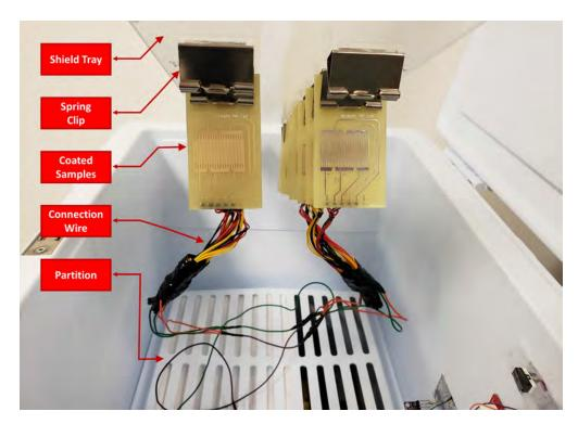
**Fig. 6.3:** Boards are ready for thermal aging in the chamber. Test samples are mounted vertically on the tray and power supply connection wires are connected.
