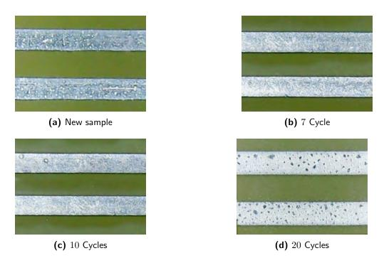
**Fig. 6.20:** Macro imaging from traces of single coated test boards with HASL finish which have degraded during 20 cycles of thermal and humidity aging under non-energized condition.
