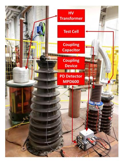
**Fig. 5.2:** Test setup for PD under pollution test. Test board is connected to high voltage source and mounted in the test cell.
