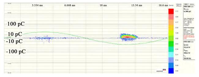
**Fig. 6.31:** Phase resolved PD pattern for a 36 cycle aged single coated test board with ENIG surface finish.
