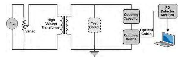
**Fig. 5.1:** PD test setup block diagram. Object under the test is connected to the high voltage transformer fed through the variac. Coupling device is in series with the coupling capacitor according to IEC60270 standard. The coupling device is connected to the measuring equipment via an optical link.
