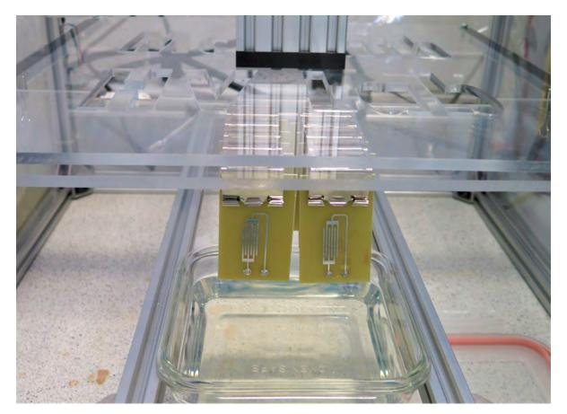
**Fig. 2.2:** PCBs mounted on the tray of conformal coating dipping machine designed and built in this research.
