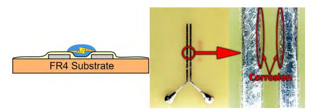
Fig. 5.6: Disruptive discharges through the contamination resulted in corrosion of the traces.
