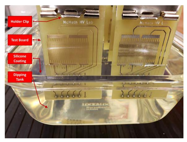
**Fig. 4.6:** Test boards are dipped in the tank of silicone conformal coating material. Boards are held vertically using spring clips.
