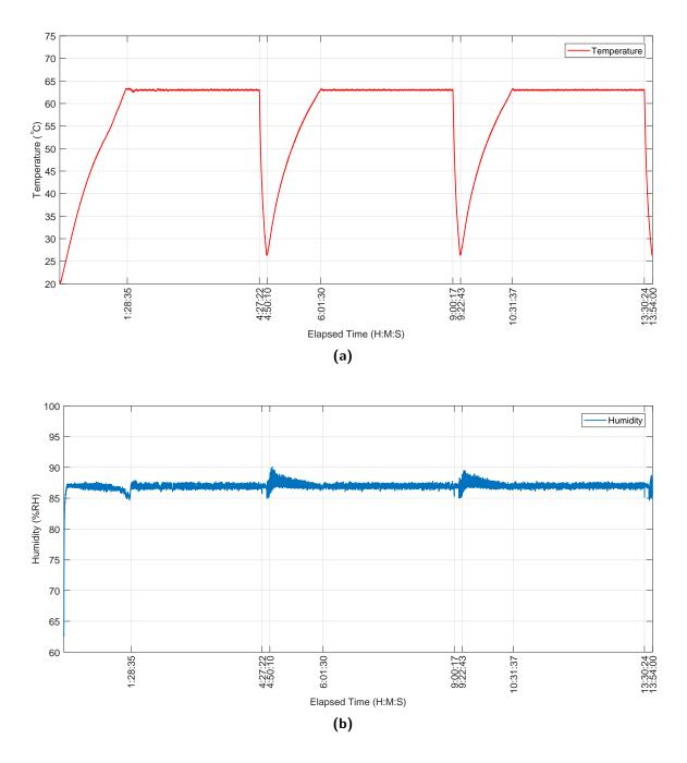
**Fig. 6.4:** Graphs of recorded temperature and humidity over three aging cycles. a) Temperature change graph in three cycles of thermal and humidity aging recorded by the chamber micro-controller unit, b) Humidity change graph in three cycles of thermal and humidity aging recorded by the chamber micro-controller unit.
