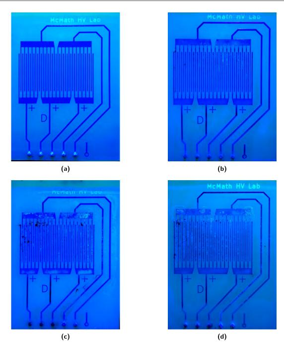
**Fig. 6.5:** Test boards under UV inspection after 36 cycles of thermal and humidity aging. Coating degradation and corrosion in traces is observed due to high humidity condition. Some blurred areas are seen on samples that show delamination of the coating layer: a) new coated sample, b) after 10 cycles aged sample, c) after 20 cycles aged sample, d) after 36 cycles aged sample.
