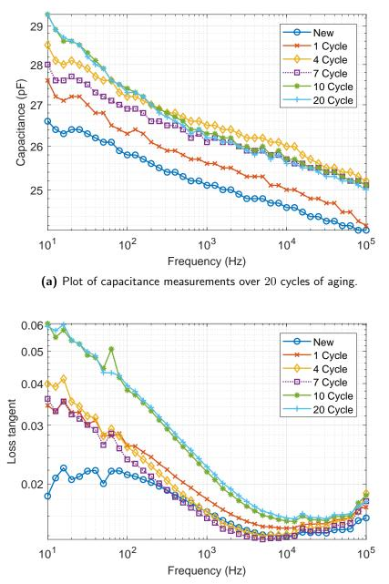
(b) Plot of loss tangent measurements over 20 cycles of aging.
