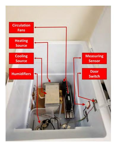
**Fig. 6.2:** Programmable thermal aging chamber setup that has been designed and built in McMath HV Lab controlled by a micro-controller.
