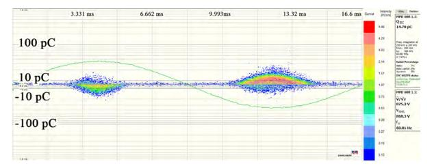
**Fig. 5.5:** Phase resolved PD pattern for coated test sample with saltwater drop on point B.
