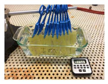
**Fig. 4.4:** Cleaning test boards by removing greasy materials from surface using isopropyl alcohol soaking for 5 minutes.
