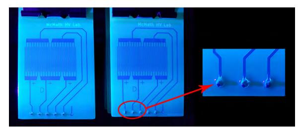
**Fig. 4.7:** Test boards under inspection using UV light. There is no issue observed on the cleaned, coated samples rather than a small boundary region around the connection pins.
