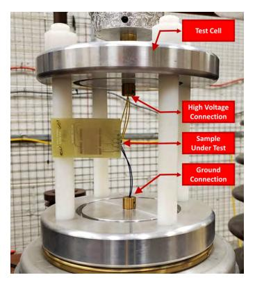
**Fig. 6.26:** Test sample mounted in the test cell and connected to high voltage source for PD testing.
