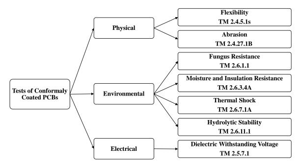
**Fig. 2.4:** Test methods for qualification of PCBs with conformal coating based on IPC TM-650 approved test methods [48].
