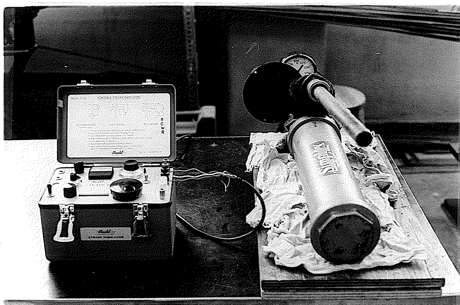
Figure 14. Pump and Load Indicating Apparatus.
