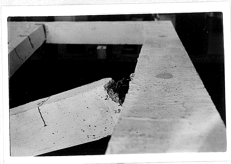
Figure 36. Broken Top Bar Near Gauge #12 Location.
