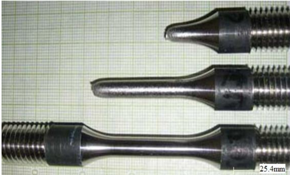
Figure 3.7 Photograph of tensile test specimen before and after fracture.
