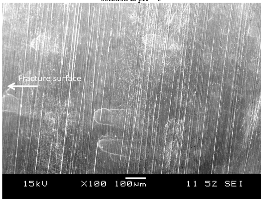
Figure 4.37 Pits near the fracture surface of IN601 after pre-corrosion formed by 10% FeCl 3 solution at pH = 0
