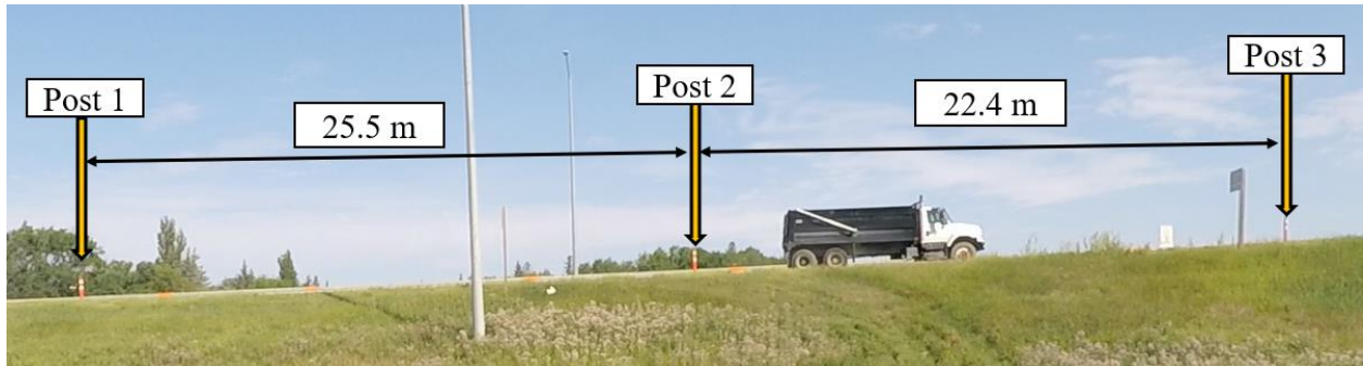
Figure 37 Image of the calibration truck and posts as visible from the field experiment camera.
