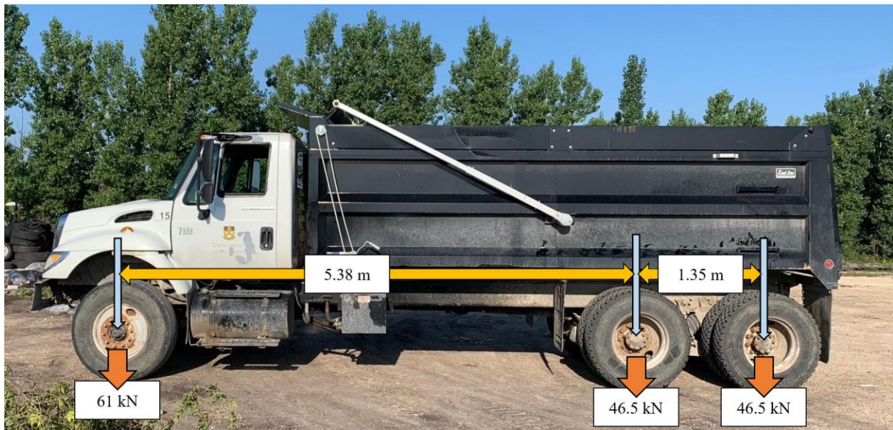
Figure 36 Image of the calibration truck for field experiment 2.
