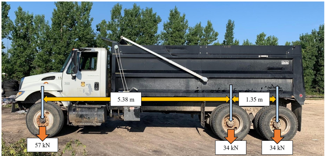
Figure 35 Image of the calibration truck for field experiment 1.
