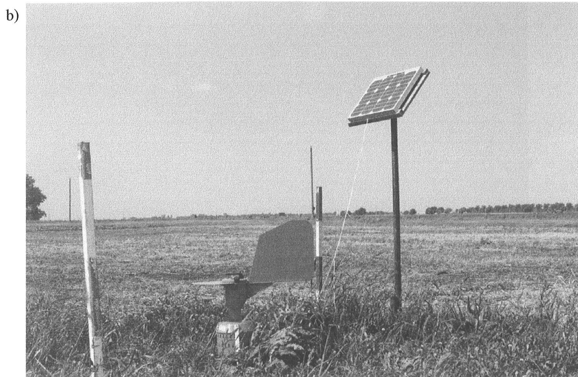
Figure 2.1: a) Rotorod spore samplers (Aerobiology Research Laboratories, Nepan, Ontario) placed at Glenlea, MB. in 1999.
