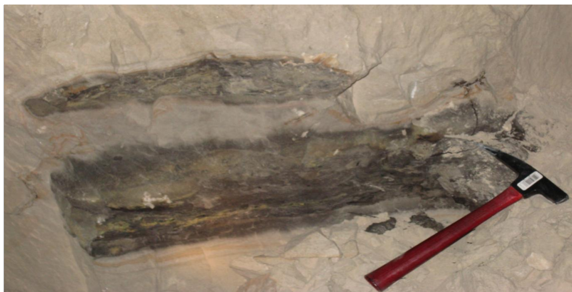
Figure 2-4: Photo of tabular sediment-hosted JD-6 uranium-vanadium deposit in underground workings. Primary minerals (coffinite, montroseite) are dark brown, grey or black. Secondary oxidized mineral carnotite is yellow and visible on working faces.
