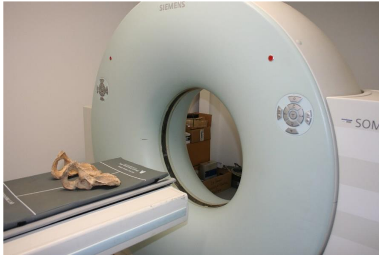
Figure 4.3: A photo of the Somatom Spirit CT scanner with an example of bone set-up (os coxae).
