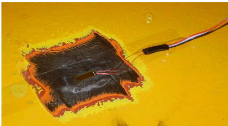
Figure 3. Strain gauge installed on wicket gate lever [3]
