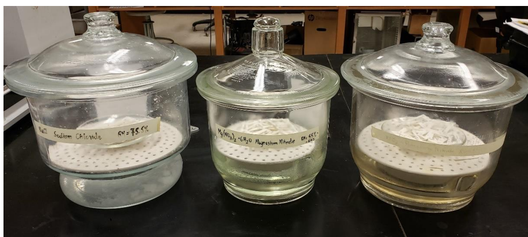
Figure 3.11 Cattail fiber kept in desiccators containing different relative humidity condition.
