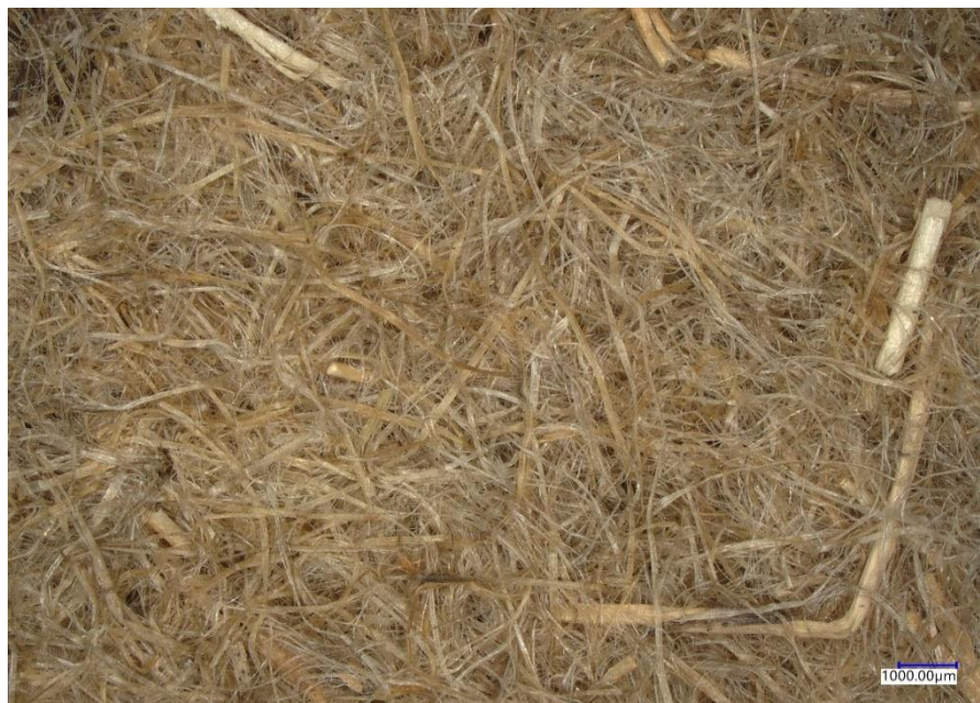
Figure 4.8 Microscopic image of 30-P flax mat at 20X magnification.
