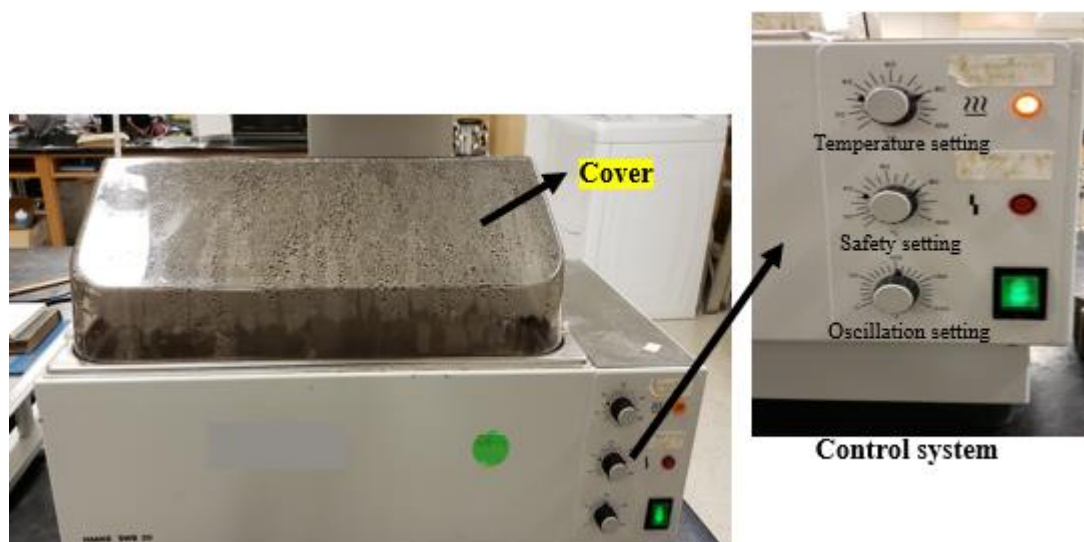
Figure 3.3 Temperature and oscillation-controlled water bath for cattail fiber extraction.
