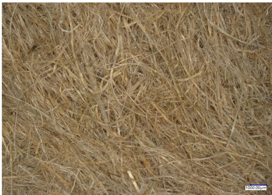
Figure 4.9 Microscopic image of 72-P flax mat at 20X magnification.
