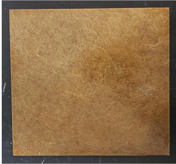
Figure 5.23 Cured cattail composite manufactured in compression molding process at 260 kPa.
