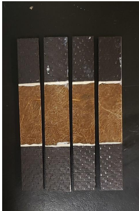
Figure 3.17 Composite specimen (127 mm X 20 mm) sandwiched between carbon epoxy laminates for tensile testing.
