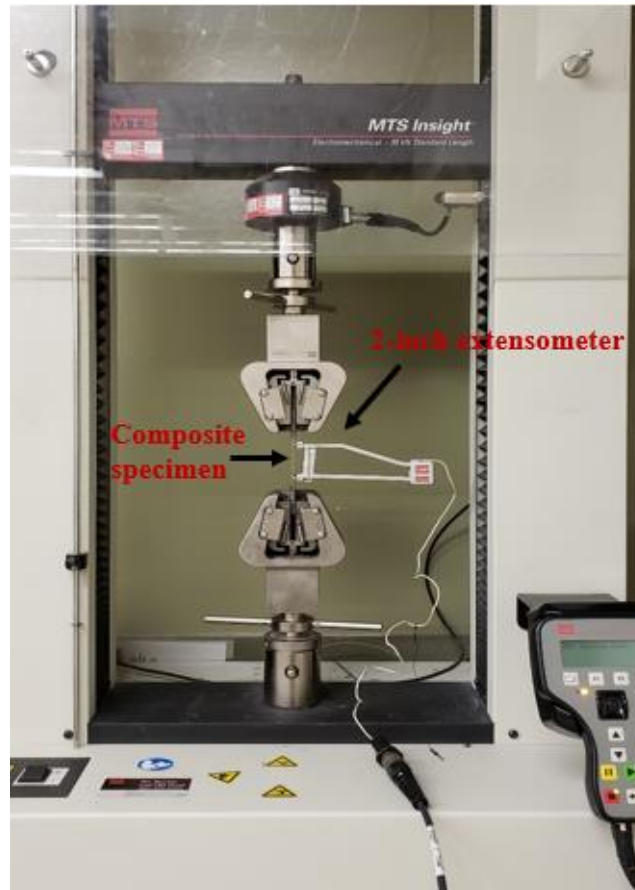
Figure 3.22 Tensile testing of composite specimens in MTS with extensometer.
