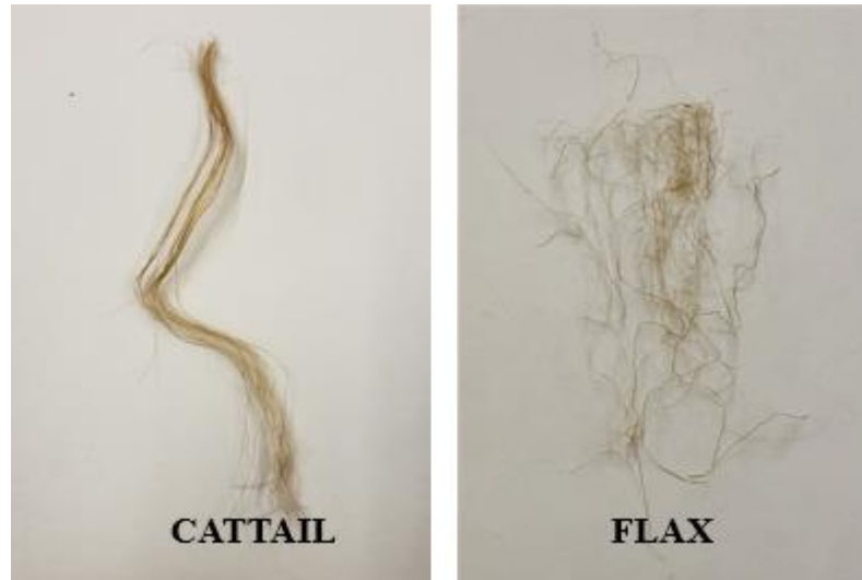
Figure 5.19 Individualised cattail and flax fiber for preparing zero punched nonwoven mat.
