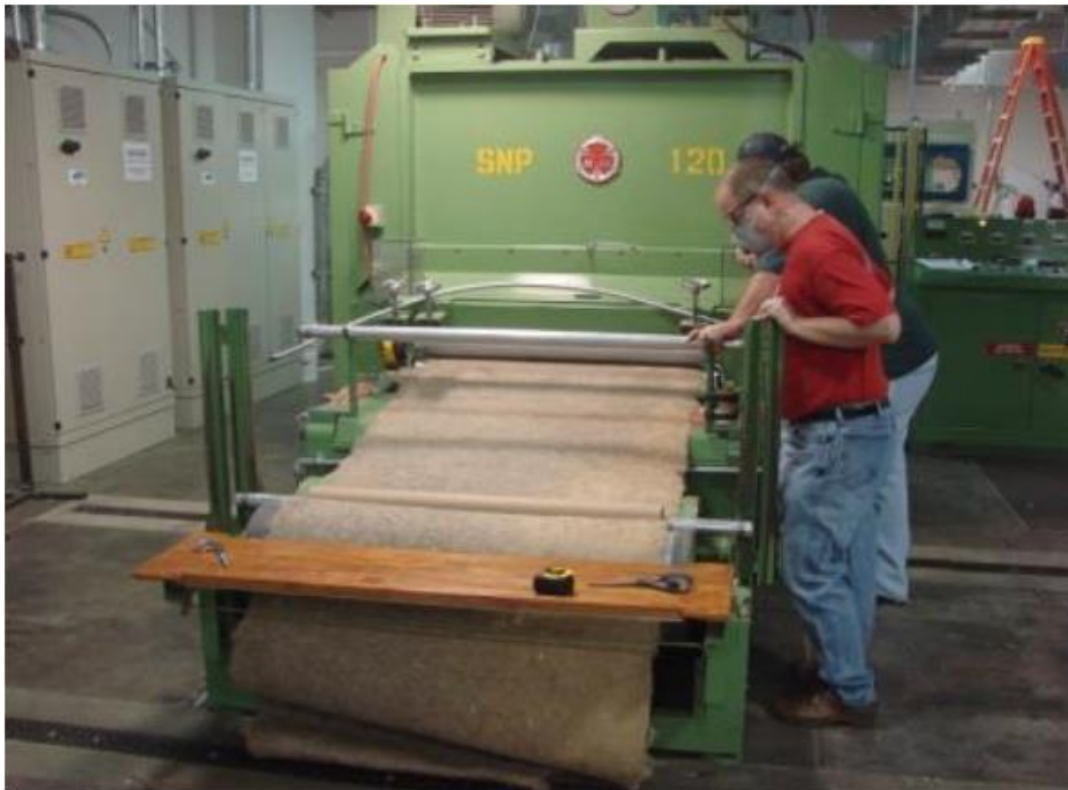
Figure 3.1 Manufacturing needle-punched flax mat (Courtesy – Dr. Raghavan Jayaraman).
