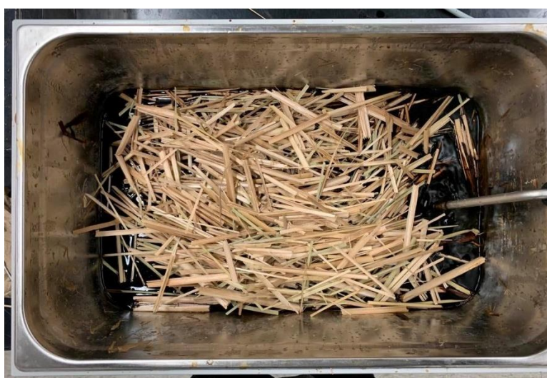
Figure 3.5 Cattail fiber extraction using reused KOH solution.
