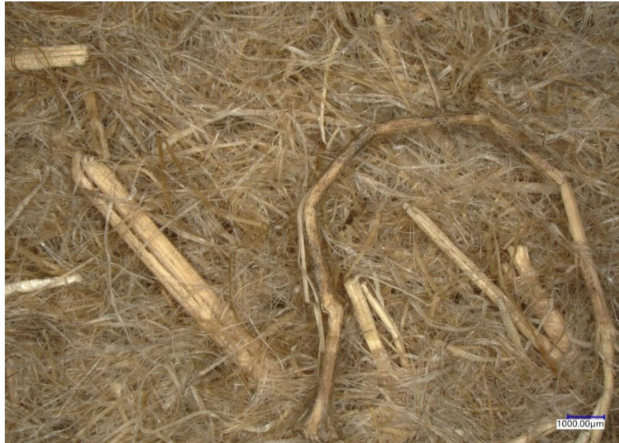
Figure 4.7 Microscopic image of 20-P flax mat at 20X magnification.
