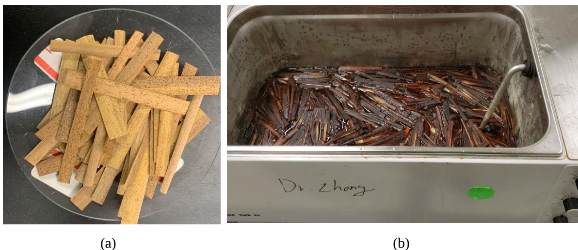
Figure 3.4 (a) Cattail plant pieces before retting (b) alkali retted cattail plant in bath after 3 hrs.
