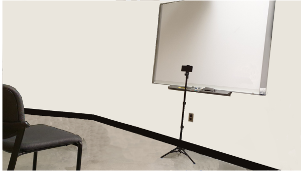
(a) Experiment Set up: Chair for user, smartphone running gesture recognizer and interaction application, and white board for projection
