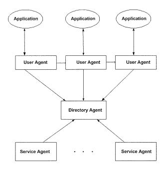
Figure 2.6: Service Location Protocol Architecture
