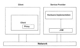
Figure 2.2: Jini Standard Architecture
