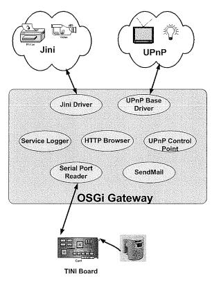
Figure 4.2: The Home Gateway Prototype
