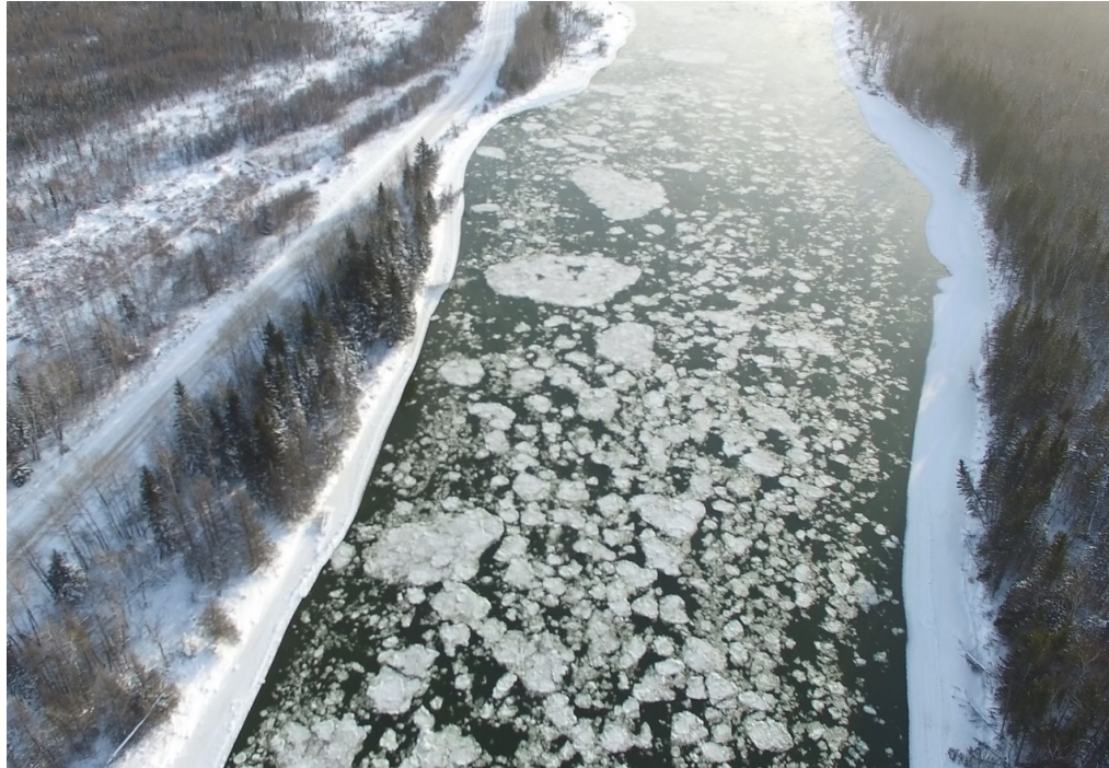
Figure 1.1. Aerial photograph of frazil slush, pans, and floes forming during freeze-up on the Dauphin River. View is looking downstream. Photograph taken on the Dauphin River on December 14, 2016.
