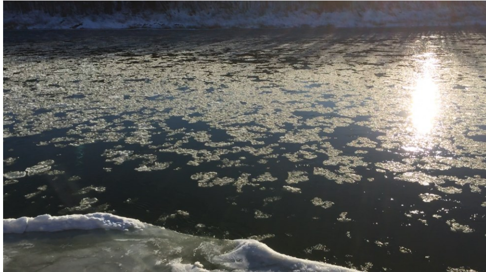
Figure 4.32. Appearance of surface ice at site DRLL05a on November 21, 2017. Note the loosely solidified frazil pans.
