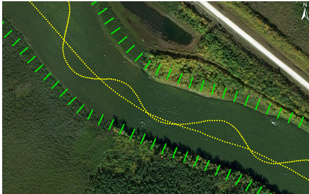
Figure 4.22. Bathymetry sources for full dynamic model. Yellow points are from bathymetric survey performed by KGS Group in 2011 and green points are interpolated bank profiles surveyed in 2016.
