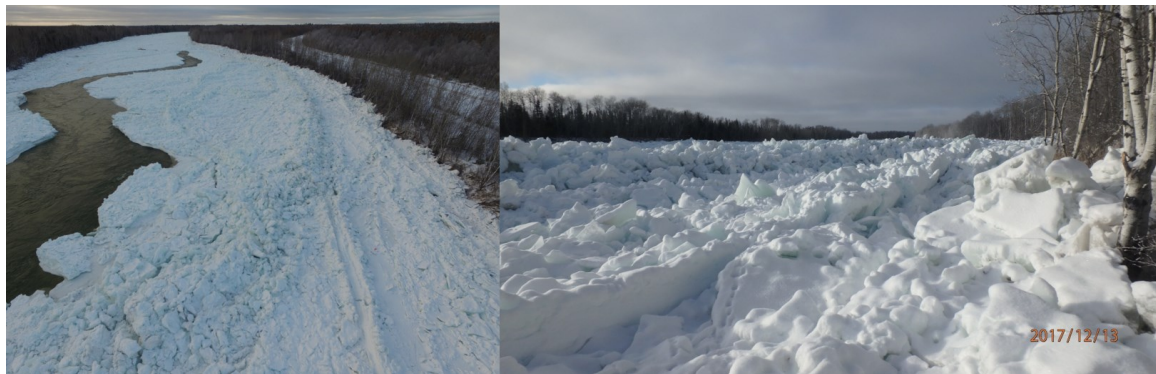
Figure 2.29. Ice cover appearance at site DRLL06 on December 13, 2017. Left photograph was taken with the UAV looking upstream. Note the ice ridge on the right side of the image. Right photograph is taken from the bank, also looking upstream.
