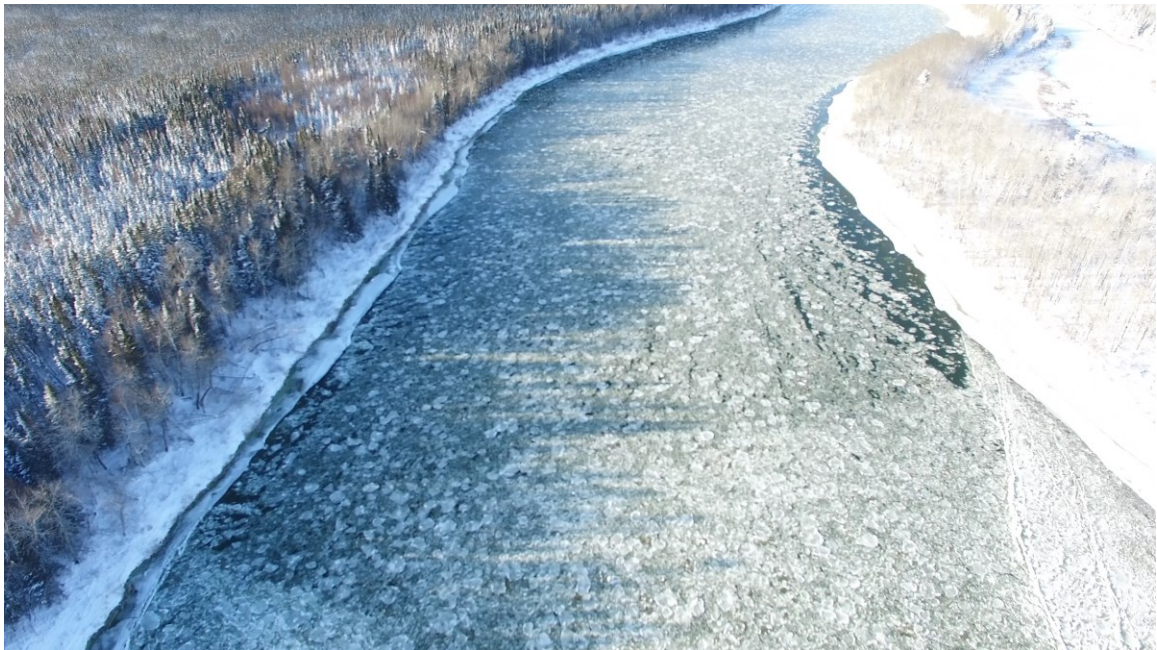
Figure 4.31. Photograph of moving surface ice at site DRLL05 taken on December 12, 2016. Flow is from top to bottom. The top portion of the image shows surface ice that is moving at a higher velocity than the ice at the bottom of the image. The convergence of the surface ice creates a moving surface layer with nearly 100% surface concentration, shown at the bottom of the image.
