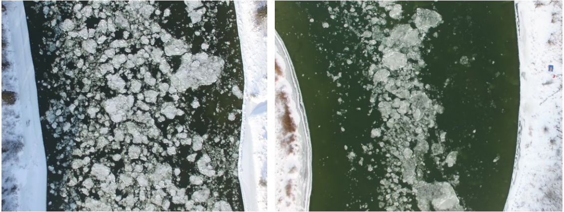
Figure 4.25. Snapshot of surface ice floes near DRLL03 taken with unmanned aerial vehicle on December 14, 2016 (left). Concurrent air temperature was -21.7^{\circ}\text{C} . Flow is from top to bottom. Average width of river is approximately 77 m. Right image shows the surface ice floes on November 21, 2017 (concurrent air temperature of -11.9^{\circ}\text{C} ) for comparison.
