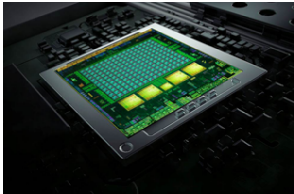
Figure 3.3: Nvidia's Tegra K1 APU which uses ARM CPU cores and their own Kepler GPU for high performance per watt at a low cost point (Smith [2014]).
