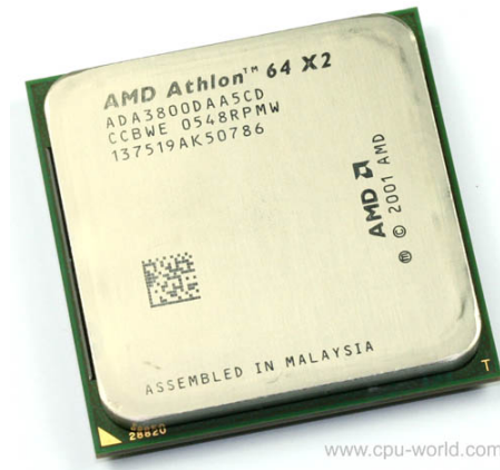
Figure 2.1: The Athlon X2, the world’s first consumer level, and AMD’s most successful, multi-core CPU, which was first shown in August of 2004 (AMD [2004]). Picture taken from CPU-World.com (Shvets [unknownb]).
