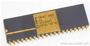
Figure 2.2: Intel’s 8087 floating point coprocessor which could be paired with the CPU to improve compute capabilities on floating point arithmetic. Image taken from (Shvets [unknowna]).
