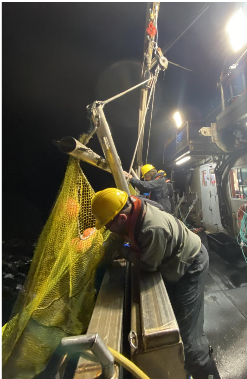
Figure 26. Benthic beam trawl being prepared for a night deployment. (Photo credit: Dr. Brynn Devine, Oceans North)
