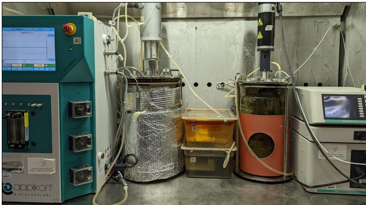
Figure 8.1 Thermophilic (TD) and mesophilic (MD) anaerobic digesters. The temperature of the TD (left) was maintained with a heating jacket and a extra layer of foil bubble wrap.
