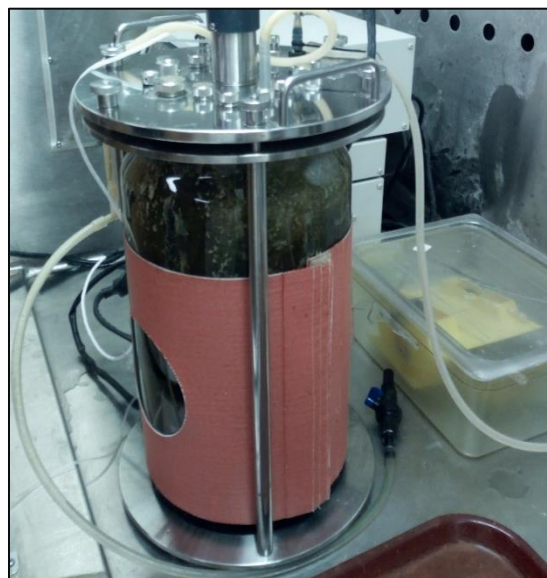
Figure 3.2 Operating mesophilic anaerobic digester.
