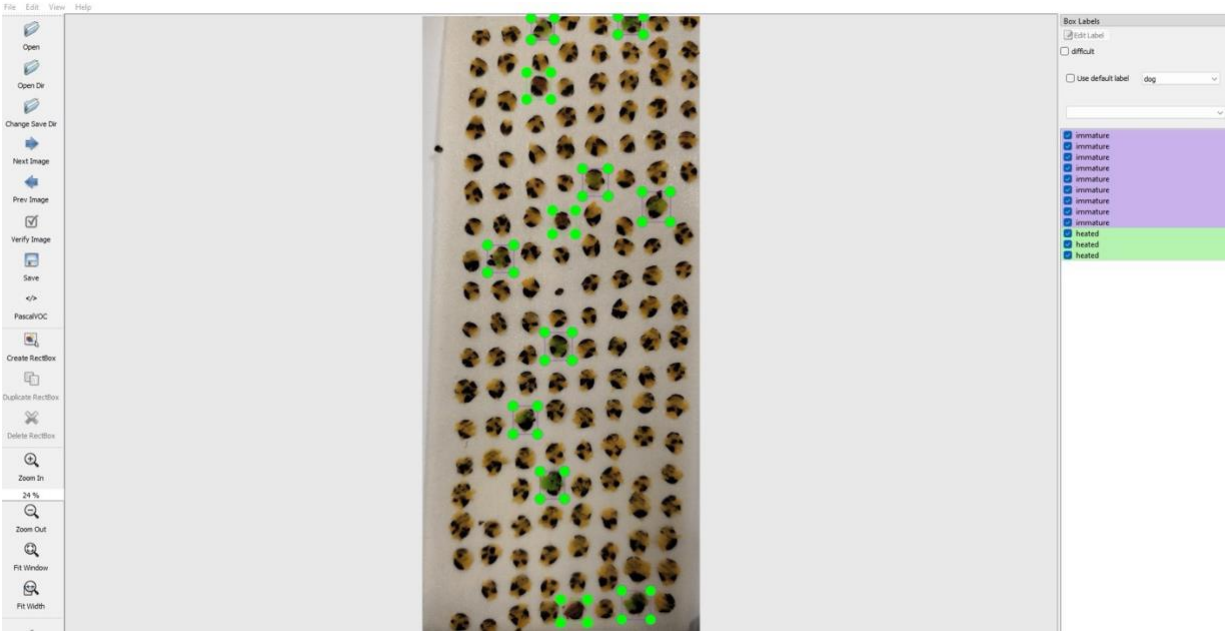
Fig. 2. 3. Data labeling using LabelImg graphical user interface. Tight bounding boxes for the two classes were drawn over the damages present to set the ground truth.
