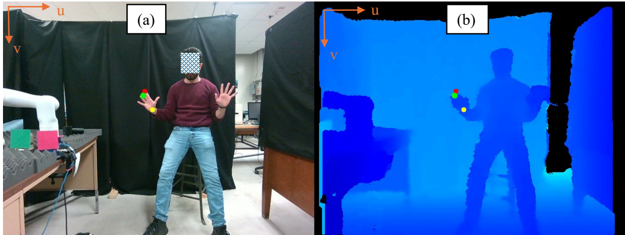
Figure 5.8: (a) RGB frame, and (b) Corresponding depth frame used as inputs to the system.
