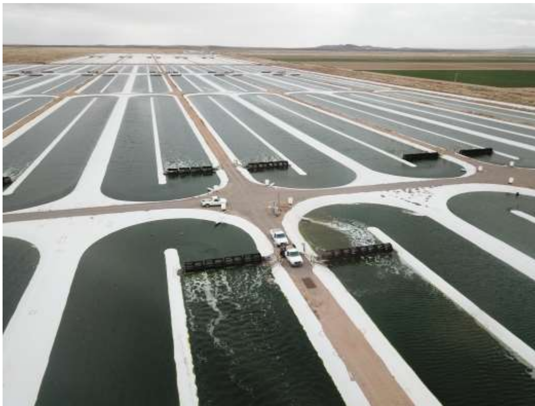
Figure 3 – High-rate algal pond ( https://www.energy.gov/eere/bioenergy/algal-production )
