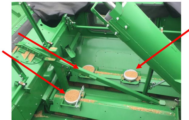
Figure 4. Three load cells mounted in the clean grain tank of 2018 John Deere S790 combine harvester. Load cells are identified by red arrows.
