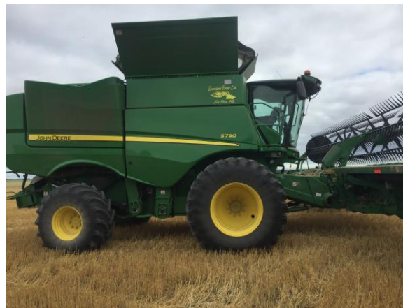
Figure 2. 2018 John Deere S790 combine harvester with open hopper top and flex draper header attached.
