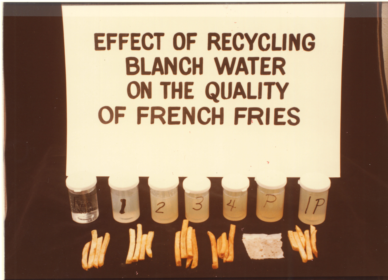
FIGURE 32. Water samples and potato french fry samples produced after 0, 1, 2 and 3 blanches and 1 primary purification treatment.
