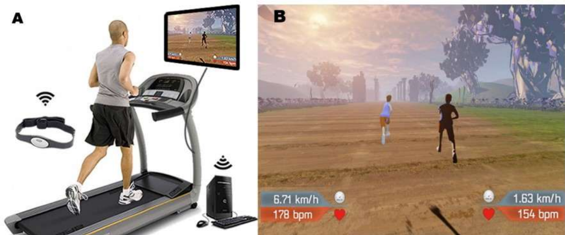
Fig. 2-1: A) setup utilized for exercising while playing, B) The game scene of two players running [27].
