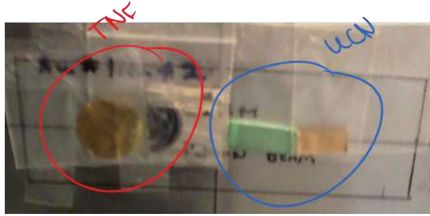
Figure 10.6: Placement of foil samples on the TNF plate. From left to right: bare TNF foil, Cd-covered TNF foil, Cd-cover UCN foils, and bare UCN foil.
