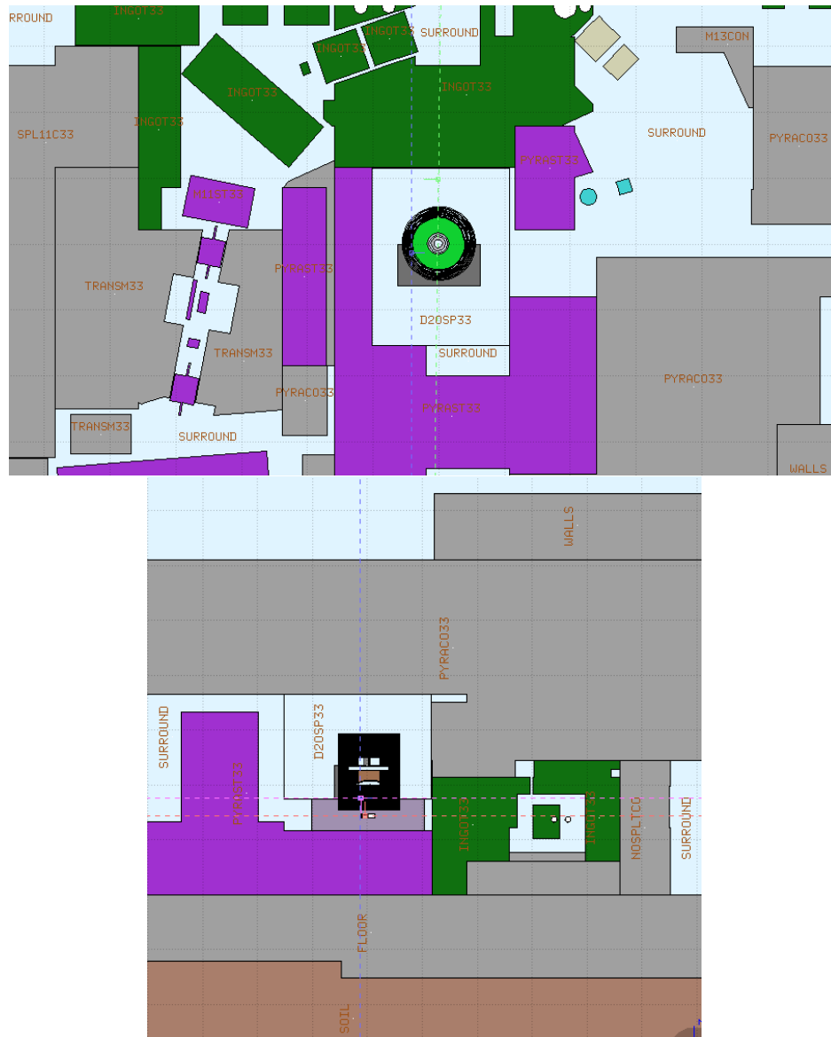
Figure 11.2: Vertical (top) and horizontal (bottom) cross sectional drawings of the cryostat and surrounding shielding in FLUKA model. The cryostat is covered with BIASING here for computing purposes.
