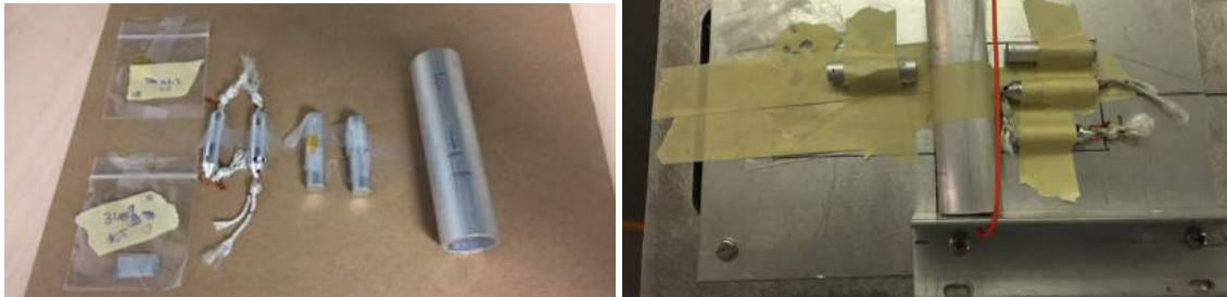
Figure 13.8: The photograph on the left shows the different samples that were irradiated in the tests (top left is a bare flat foil, below that is a Cd covered foil, then from left to right is a gold foil in an Al boat, Cd covered gold foil in an Al boat, gold foil on an Al bar, Cd covered gold foil on an Al bar, and finally inside the Al pipe there is a bare foil on Al rod, and a Cd covered foil on an Al rod. The panel on the right shows the arrangement of these samples on the TNF sample holder. The black rectangle in pen on the Al irradiation plate is the region of uniform neutron flux.
