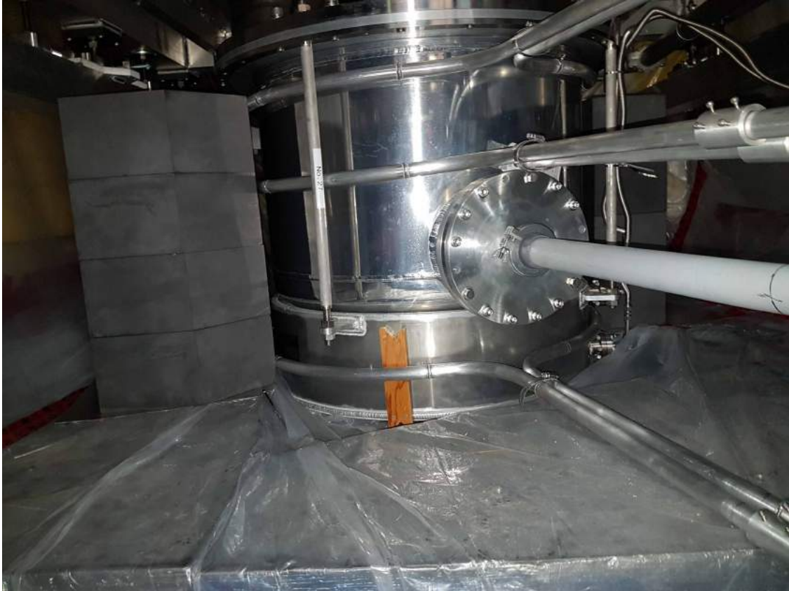
Figure 12.2: Photograph of cryostat with pipes for foil placement and the surrounding graphite columns. Only one column of graphite is seen here, but there were three columns for the measurement.
