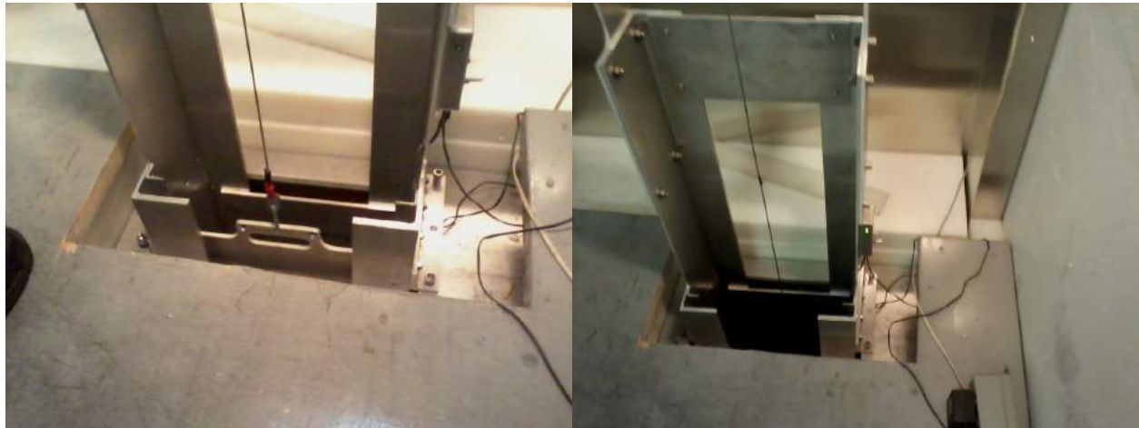
Figure 10.7: Lowering TNF plate into thermal neutron beam. The TNF plate is attached to the pulley and then lowered until the green light illuminates (seen in second figure). This ensures that the plate is placed in the correct position for uniform beam.
