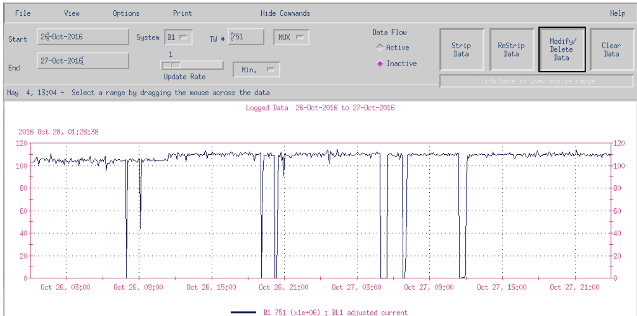
Figure 10.8: Current (in \mu\text{A} ) from the cyclotron before, during, and after the irradiation.
