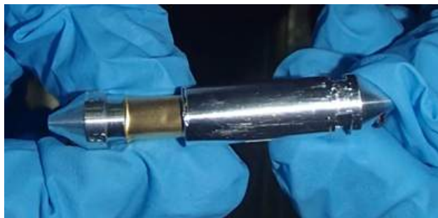
Figure 12.1: Photo of the Al boat used for placing the Au foil around the cryostat. The boat is in the open position in order to show the foil wrapped inside.
