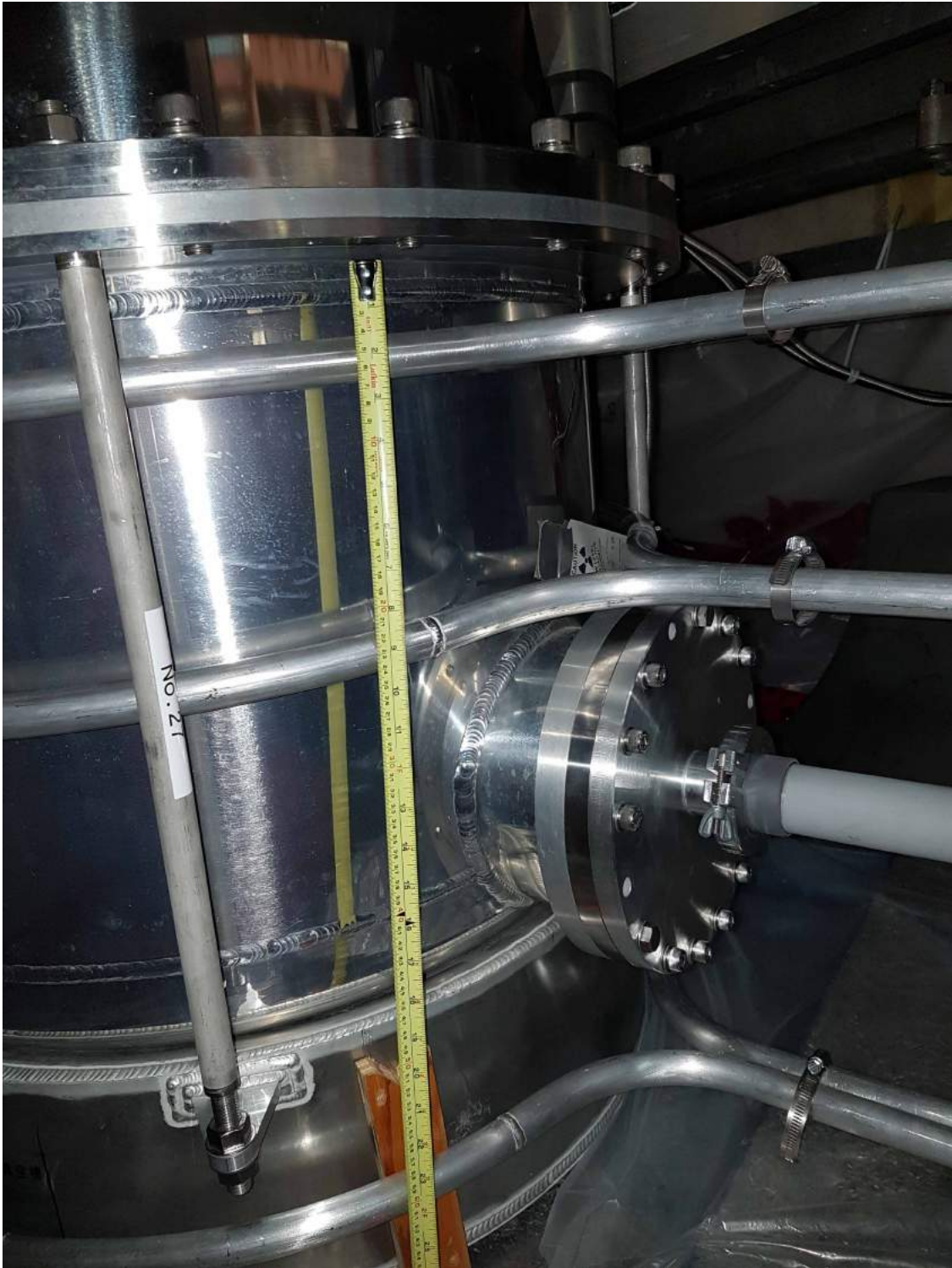
Figure 13.1: Photograph of the cryo area of the cryostat. The pipes for foil placement are situated around the outside of the cryostat. The welding line shows the transition between the warm volume and the cold volume.
