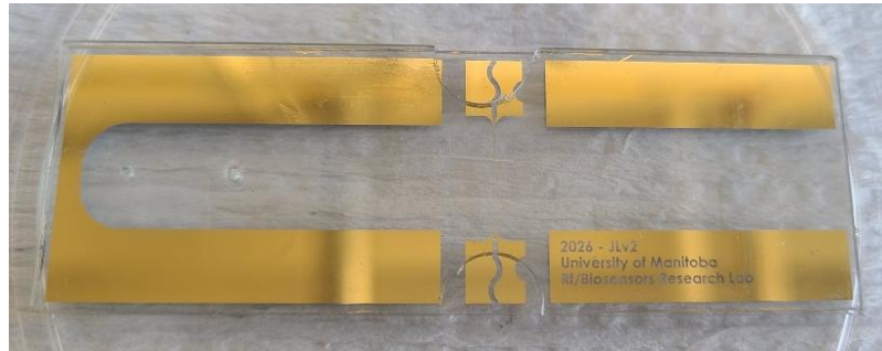
Figure 3-5: Fabricated microfluidic channel with integrated DEP electrodes.
