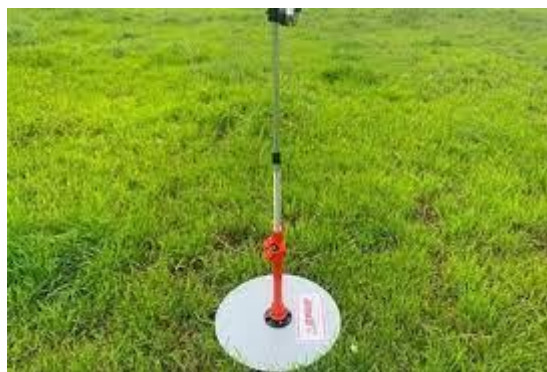
Figure 3.1. The rising plate meter (RPM) is a common tool for grassland AGB estimation (Rankin & Komainda, 2023).
