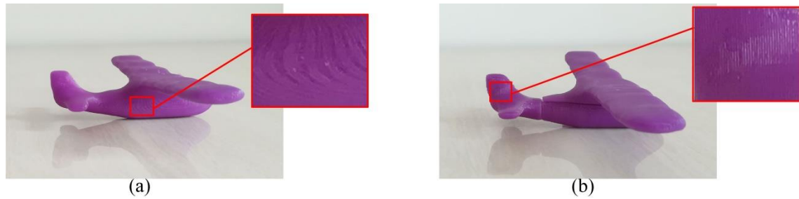
Figure 6-19 Surface quality of printed models
