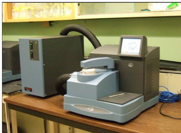
Figure: 3.4 DSC Q200 equipment used for critical temperature analysis.
