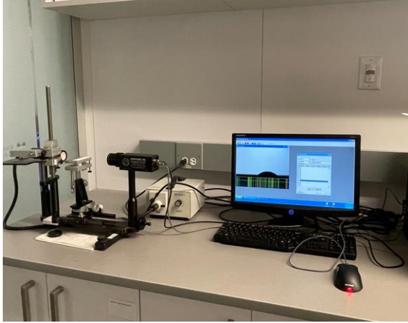
Figure 3.6 Ramé-Hart Inc., Model 200-00-115 used for water contact angle measurement.
