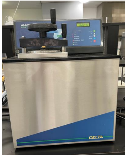
Figure: 3.2 ANKOM fibre analyser used for chemical composition analysis (cellulose, hemicellulose and lignin).
