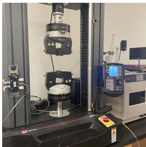
Figure: 3.8 Instron instrument used in measuring tensile strength.
