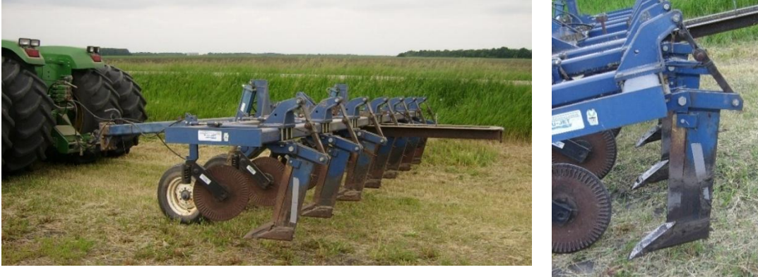
Figure 2.1. A subsoiler with wavy coulters and rippers.
