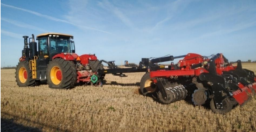
Figure 2.1. Example of disc equipment that managing soil and crop residue (designed and manufactured by Versatile).
