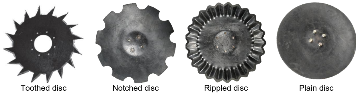
Figure 4.1. The illustration of different types of disc tillage tools, toothed disc referred to Bianchini and Magalhães (2008).
