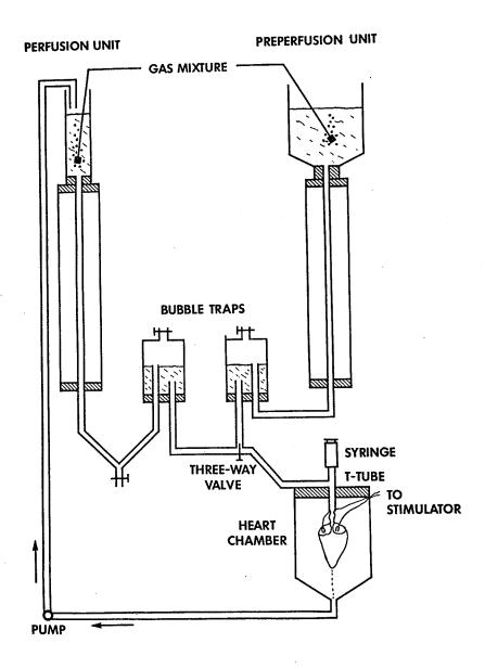
Figure I. Schematic diagram of the perfusion apparatus. See text for explanation.
