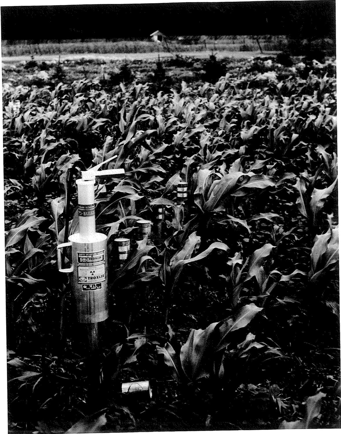
Figure 4.3 Photograph of Moisture Gauge Fitted on the Top of Access Tube
