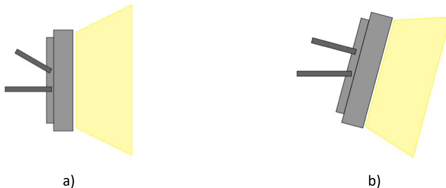
Figure 19 - Proposed lighting change. a) side lighting used for experiment b) proposed angled lighting for future testing
