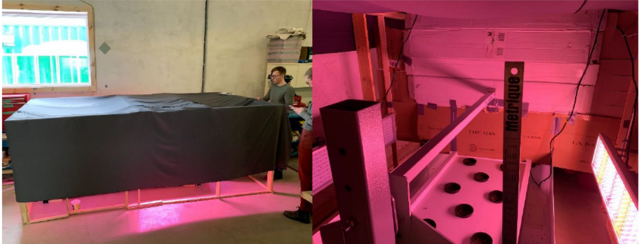
Figure 11 - Frame with blackout fabric over it (left), and light divider between side and top lighting halves (right)
