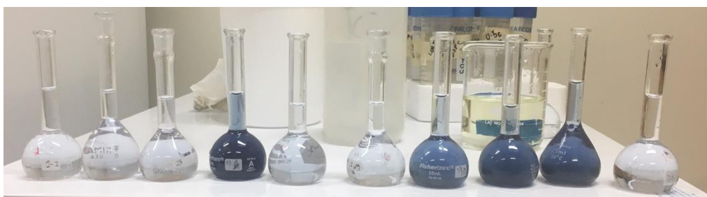
Fig. 5 Samples of zebra mussel shell treated phosphorus water, with ascorbic acid method reagent b. Source: The author.
