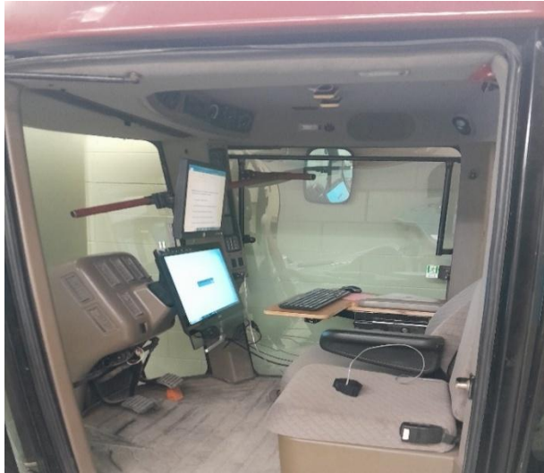
Fig. 4.1. Tractor cab used for the experimental study. Participants used the upper monitor for the internet search task while the lower monitor displayed the simulation of the autonomous agricultural sprayer.
