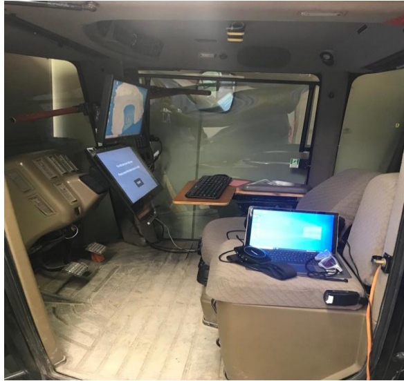
Figure 5.1. Tractor cab used for the experimental study. Participants used the upper monitor for the internet search task while the lower monitor displayed the simulation of the AAMs.
