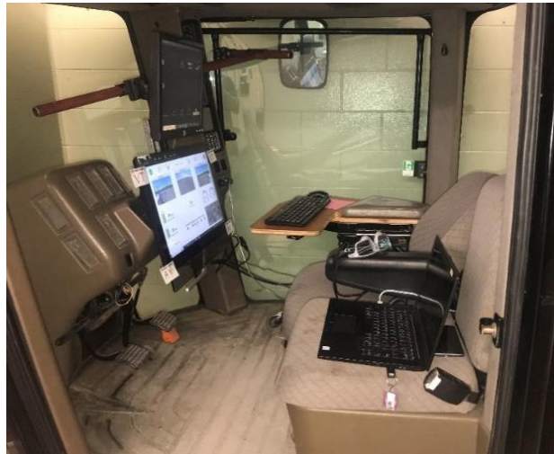
Figure 3.1 A tractor cab was used for the experimental study. Participants used the top monitor for the internet search task, while the bottom monitor displayed the simulation of the autonomous agricultural sprayer.
