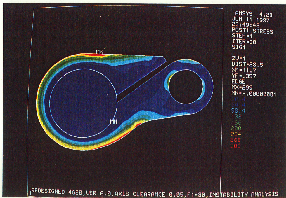
Figure D17(b) : Principal Stress Distribution, R=0.05\text{mm} , W=2000\text{N} .
